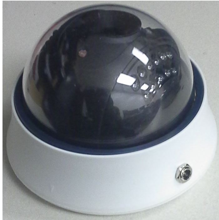
Figure 2.2: The camera housing used to hold the smart-camera's RPI2 and camera module[2]
