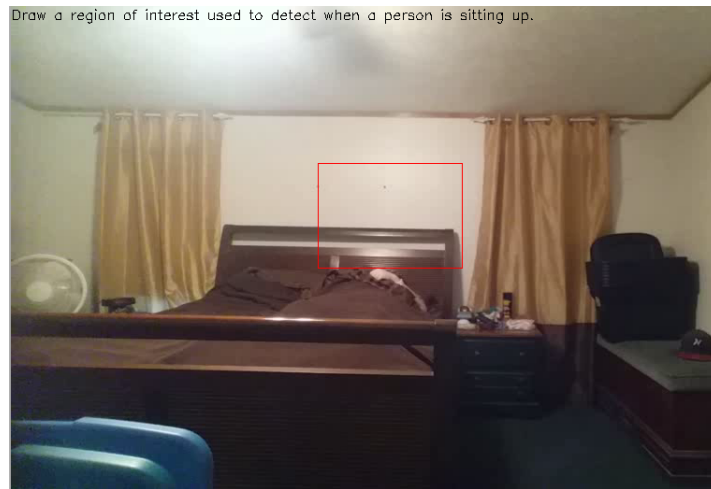
Figure 3.9: An example of where to place a sitting-up region. The region is enclosed in the red rectangle. It is above the person lying in the bed.
