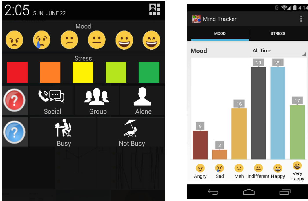
Figure 6.1: Application UI. Left: Notification-only UI for collecting training data. Right: Mood data visualization.
