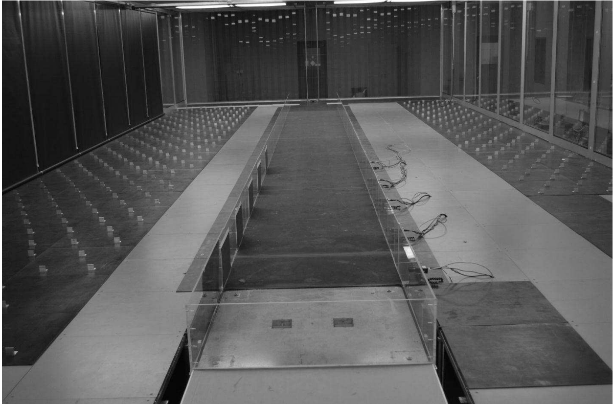
Figure 3.6 A view looking down the channel from behind the box. Note that in this photo the lid is not covering the box (as opposed to Figure 3.4) and the moving floor is at the top position. (Photograph by author)
