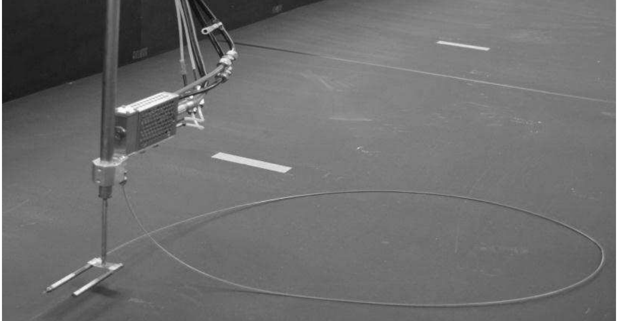
Figure 3.8 Photograph of the sampling tube, HSM, and measurement arm. (Photograph by author)
