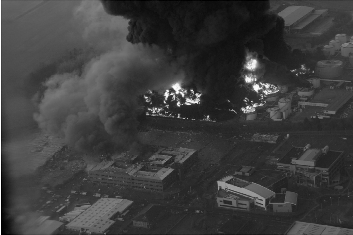
Figure 1.1 Photograph of the Buncefield site [4] in the immediate aftermath of the explosions. The nearly straight fire line is the western wall of the dike which contained the overfilled tank. Between this dike and the smoldering structure is the parking lot where the largest explosion took place. The fuel depot was surrounded by an office park. If the accident had taken place during normal working hours it is likely that there would have been fatalities.
