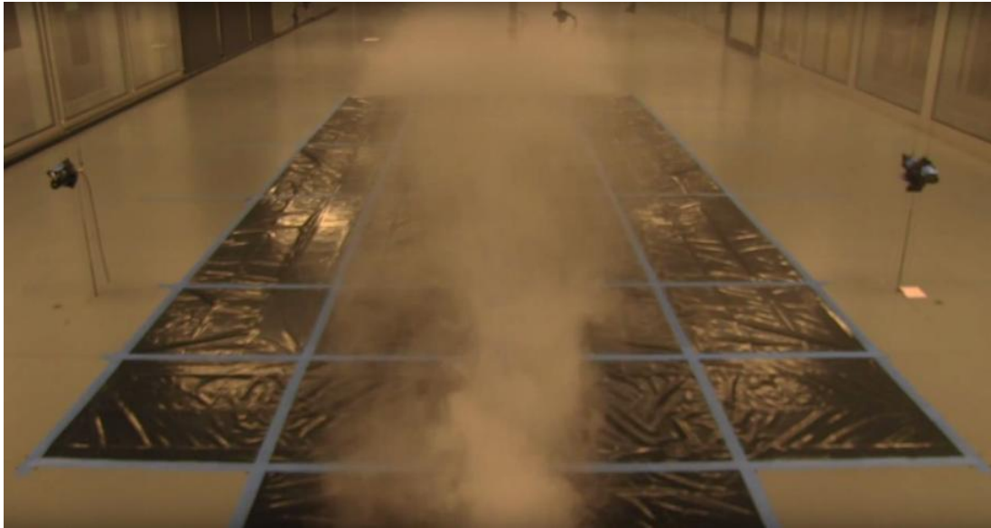
Figure 32. Uniform flow in the tunnel with fog and black plastic on the floor for visualization
