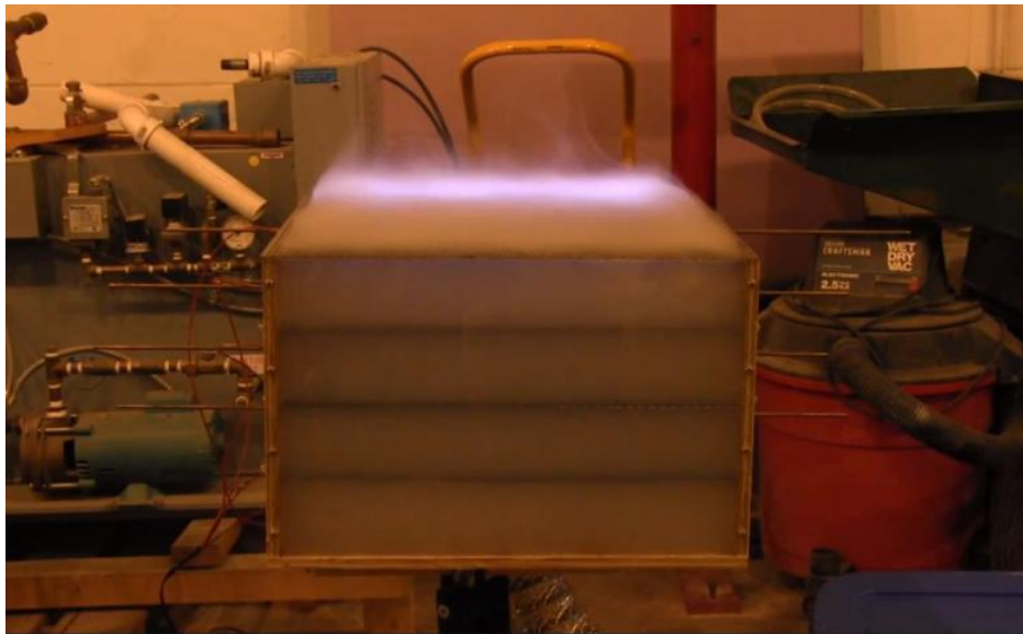
Figure 34. Screenshot of video to show well-distributed flow through preliminary area source
