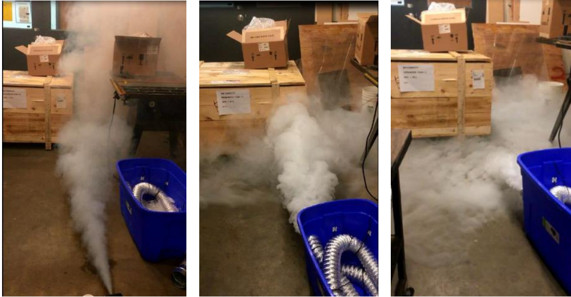
Figure 47 Delivery of 50% glycerin solution with no dryer duct (left), with dryer duct (middle), and with dryer duct submerged in ice (right)
