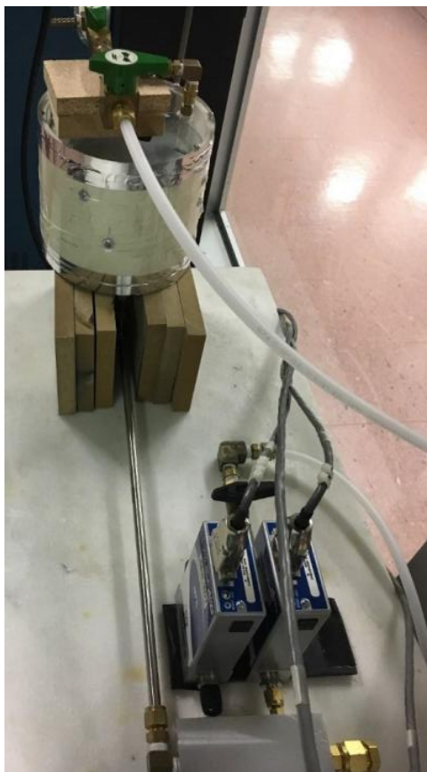
Figure 44. Dead space, static mixer, and aluminum box for accurate delivery of gases
