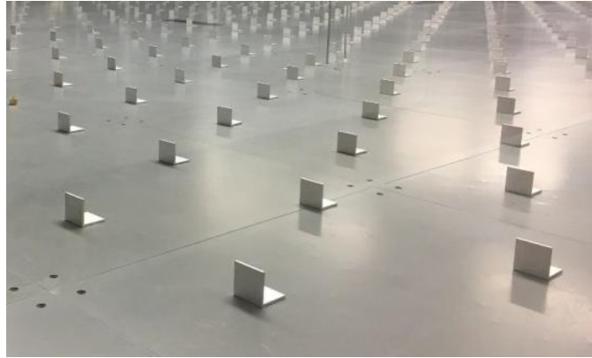
Figure 31. Physical placement of aluminum angles for surface roughness in wind tunnel
