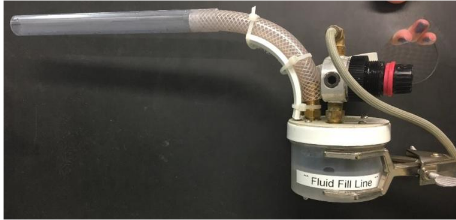
Figure 46. TSI Model 8320 Atomizer with outlet tube modifications for optimal seeding
