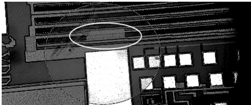
Fig. 7.3 Zoomed view of the defect under probe station (problem area is circled). (Lamichhane, Ranjan. February 2013. CSRC Lab. JPEG file.)
