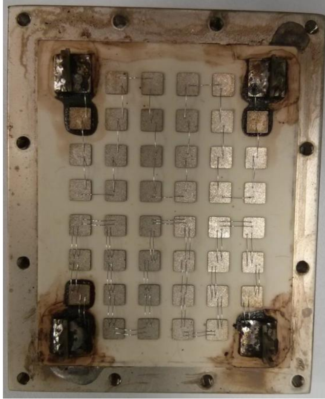
Figure 5.4(a). Un-encapsulated test module after thermal cycling
