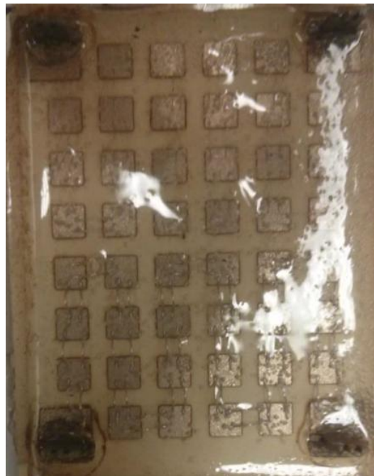
Figure 5.7. Flux cleaned and encapsulated test structure after thermal cycling
