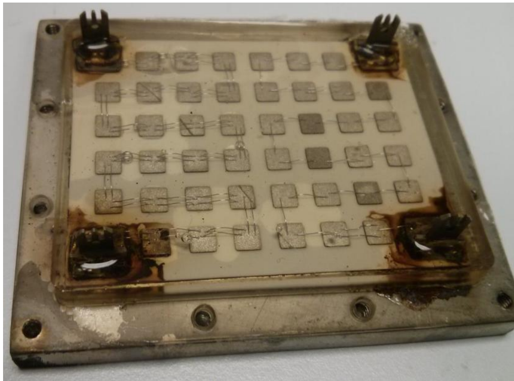
Figure 5.4(b). Encapsulated test module after thermal cycling
