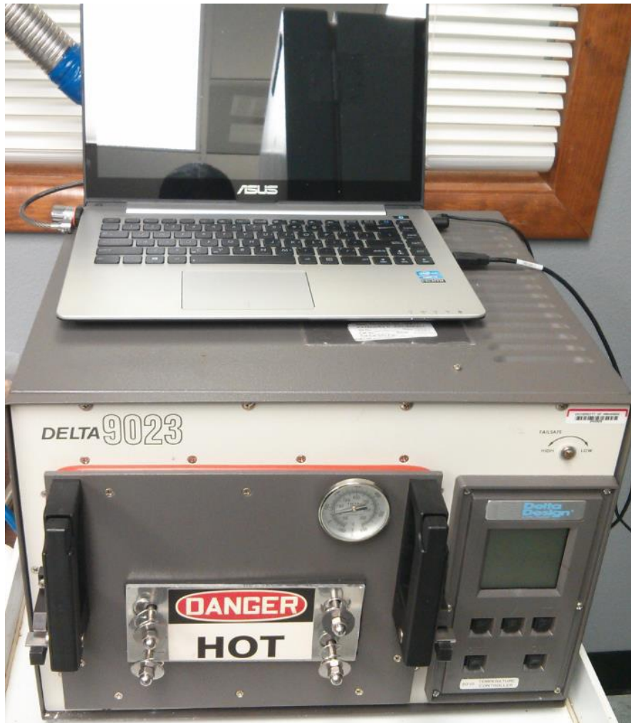
Figure 5.3: Thermal cycling furnace
