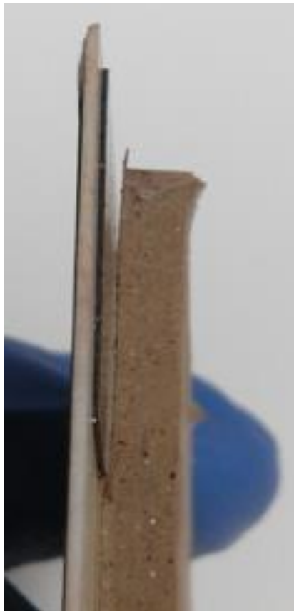
Figure 5.12. De-lamination of encapsulation from the DBC substrate
