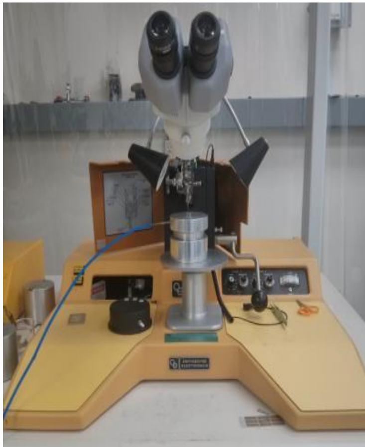
Figure 2.4. Orthodyne ultrasonic wedge bonder
