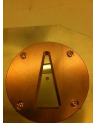
Figure 3.11 (b) Front side of loaded piece cassette (Thach Pham, January 2013, University of Arkansas)
