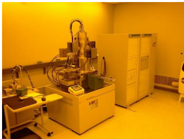
Figure 2.1 EBL JEOL 5500ZD system (Thach Pham, June 2012, HiDEC cleanroom, University of Arkansas)
