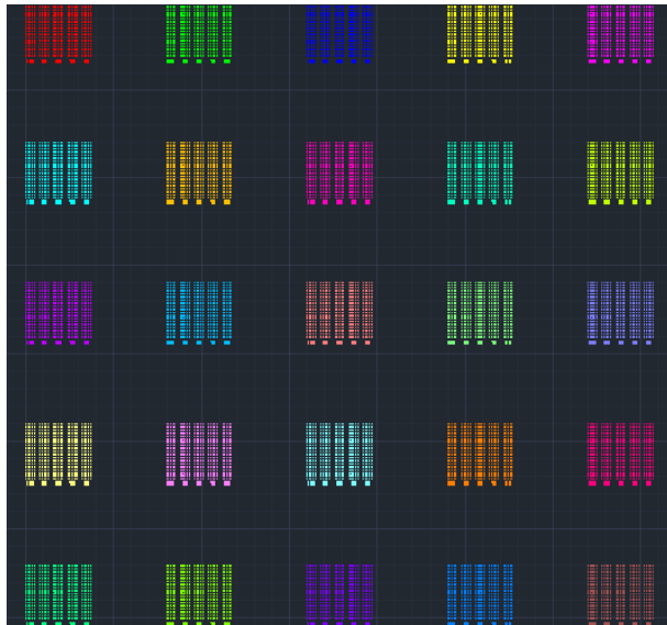
Figure 3.2 (a) CAD design 5x5 arrays of different doses (Thach Pham, December 2012, Auto CAD 2012)
