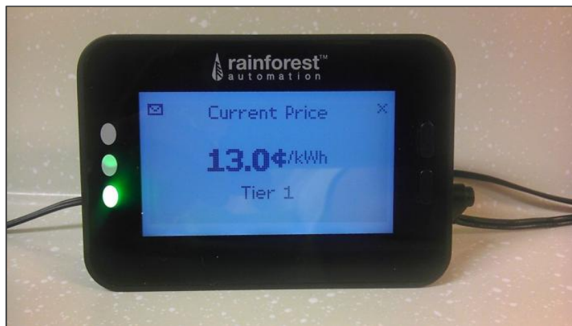
Fig. 3. A wireless mesh networked energy monitoring unit displays current pricing information for a residential consumer under the Southern California Edison electrical system. “Traffic light” style indicators on the side indicate the current pricing tier.
