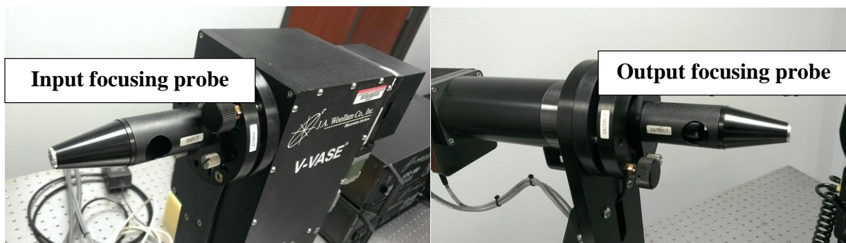
(d) Focus probes mounted on the source and detector units
