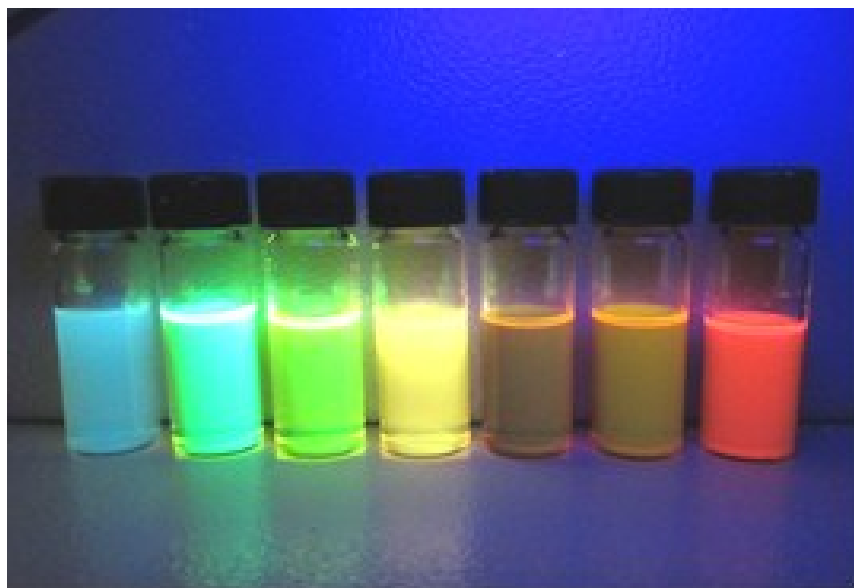
Figure 5.4 A photograph of InP/ZnS core/shell nanocrystal samples emitting from blue to red is shown.
