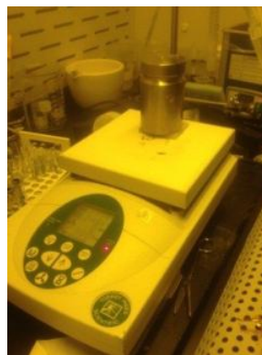
Fig. 6.16 Sintering of nano silver paste on top of a hot plate (photo by author)
