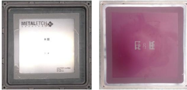
Fig. 6.14 Stencil (left) and screen (right) used for applying nano silver paste (photo by author)
