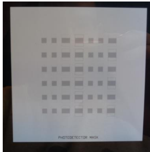
Figure 2.6 Image of the mask used in photolithograph, photo taken by the author in 6/1/2013.
