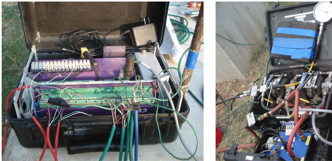
Figure 5.28. Photographs of (a) data acquisition system, and (b) automated pressure regulator and hydraulic pump utilized to perform the O-Cell testing.
