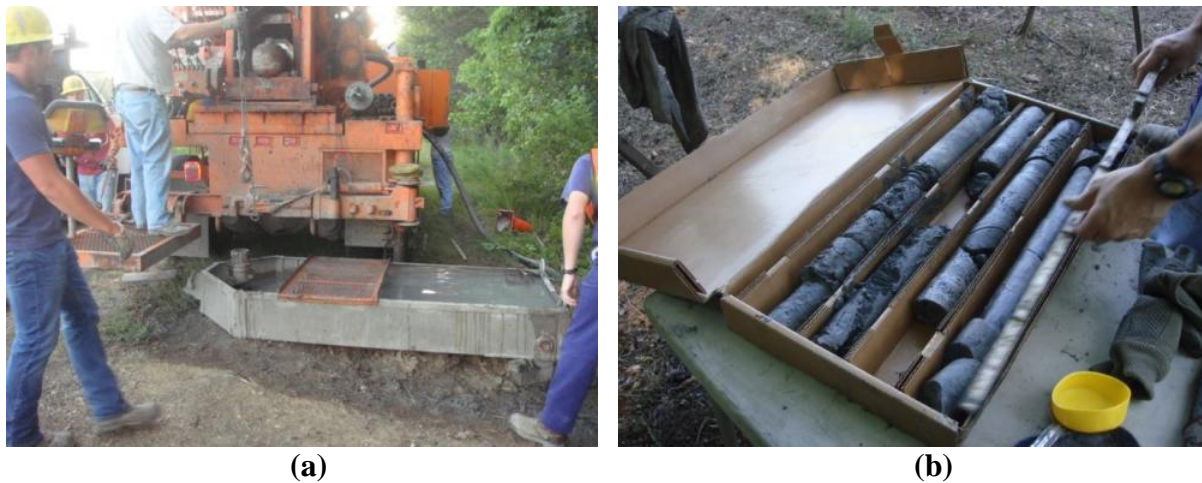
Figure 6.6. a) Changing to rotary wash method at B-6, and b) rock sample obtained from B-6.
