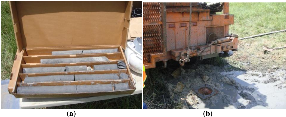
Figure 6.3. a) Rock sample obtained coring at B-2 (validation site), and b) post-drilling conditions at B-2
