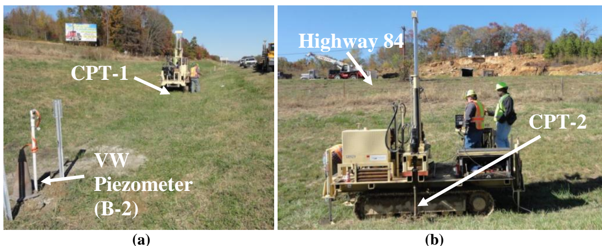
Figure 4.41. a) Cone penetrometer test being performed at the CPT-1 location, and b) cone penetrometer rig conducting the test at CPT-2 location.
