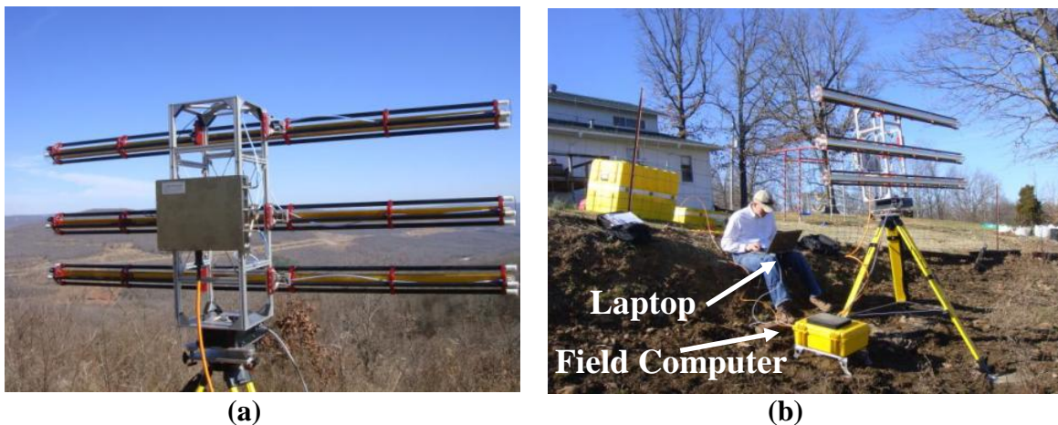
Figure 4.26. a) Viewing geometry of the GPRI-II at overlook viewpoint, and b) University researcher acquiring data with GPRI-II.
