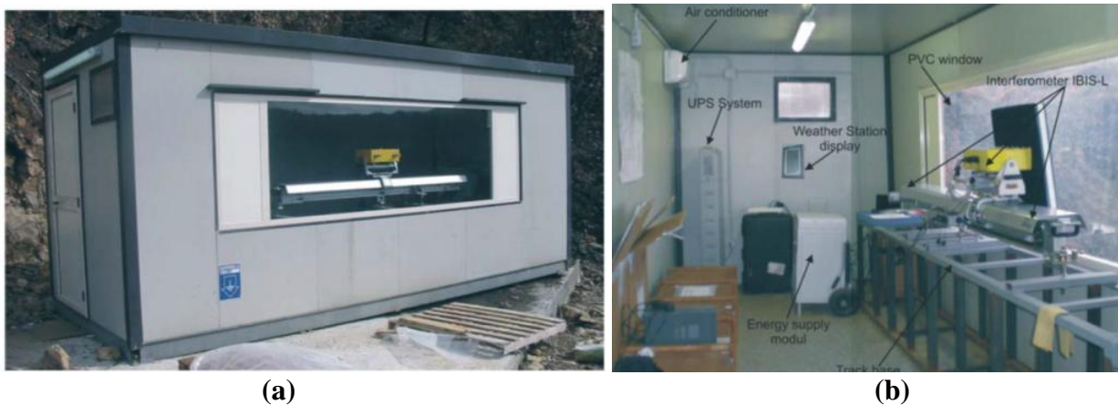
Figure 2.13. a) Photograph of the exterior of IBIS-L platform enclosure, and b) photograph of the interior of the platform enclosure including the IBIS-L system (from Bozzano et al., 2008).
