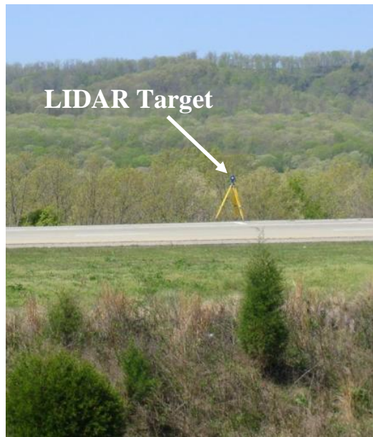
Figure 4.31. LIDAR target positioned at the Southbound Total Station viewpoint at the calibration site near Chester, Arkansas.
