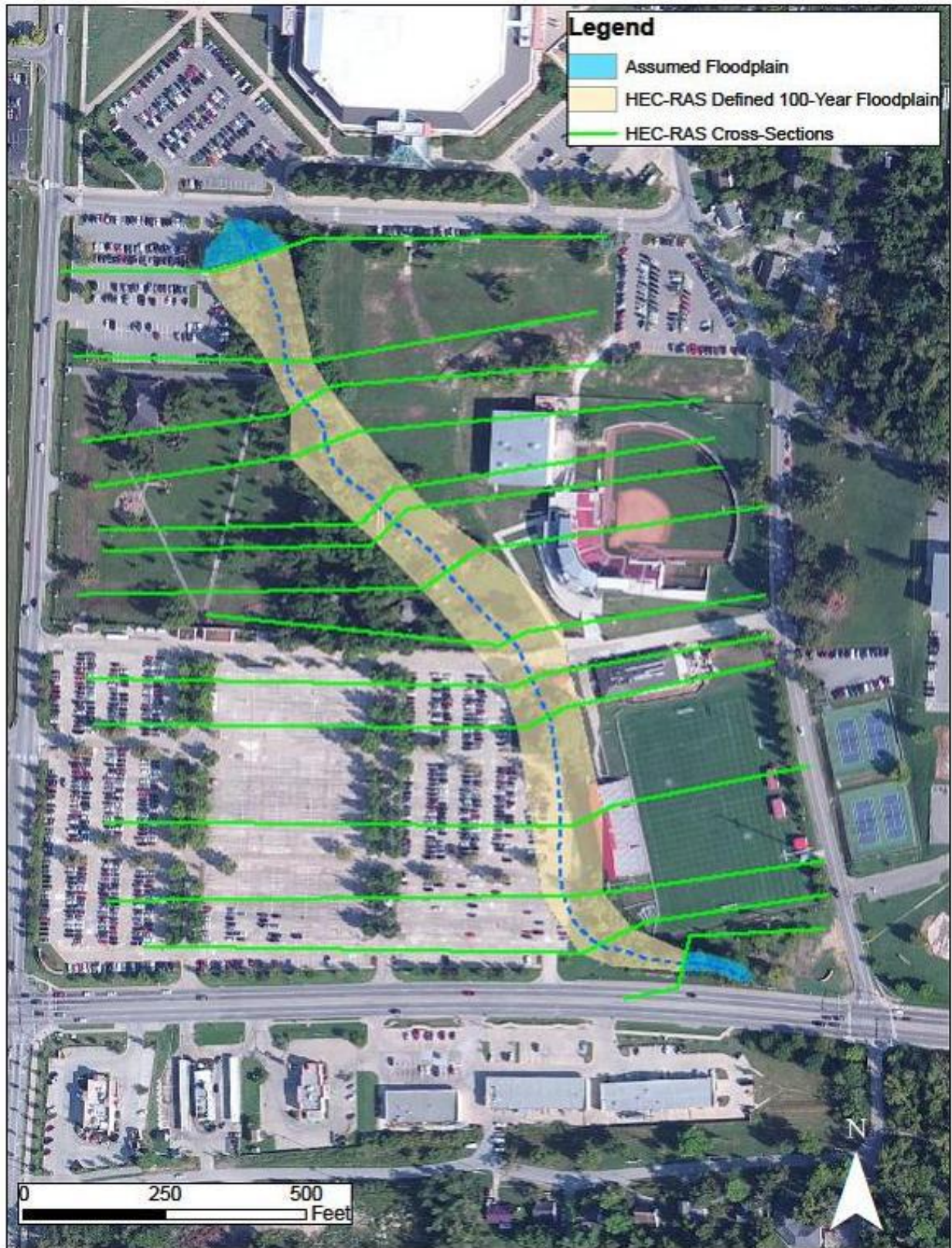
Figure S3. 100-Year Flood Boundary for Two-Stage Channel and Storage Design Conditions
