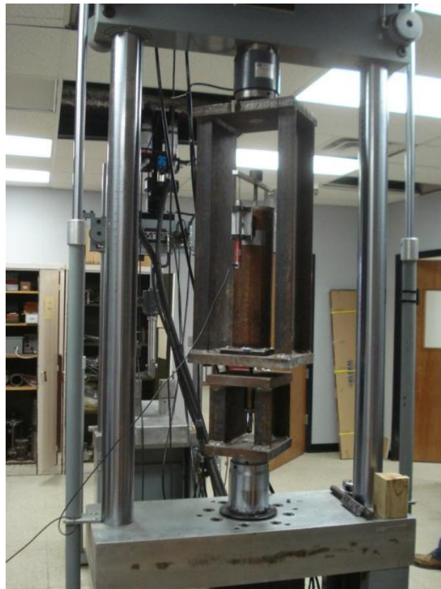
Figure 3.12: Setup for Standard Test for Strand Bond
