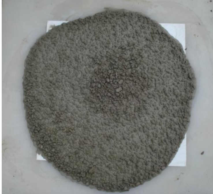
Figure 4.4: Slump flow of final NSS mixture
