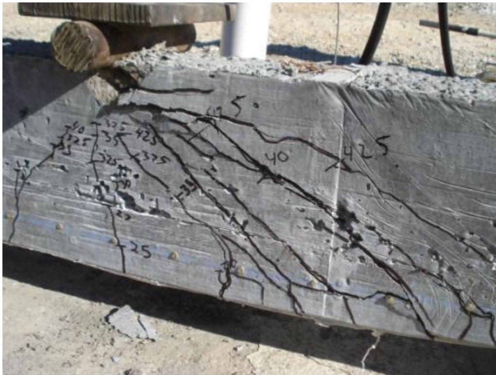
Figure 6.65: Shear failure of specimen HSC-4D
