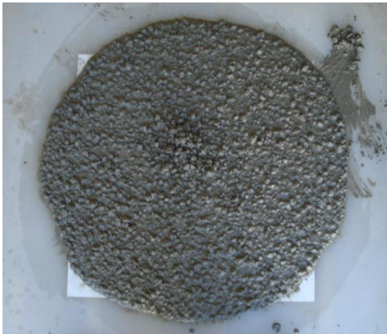
Figure 4.10: Slump flow of final HSC mixture
