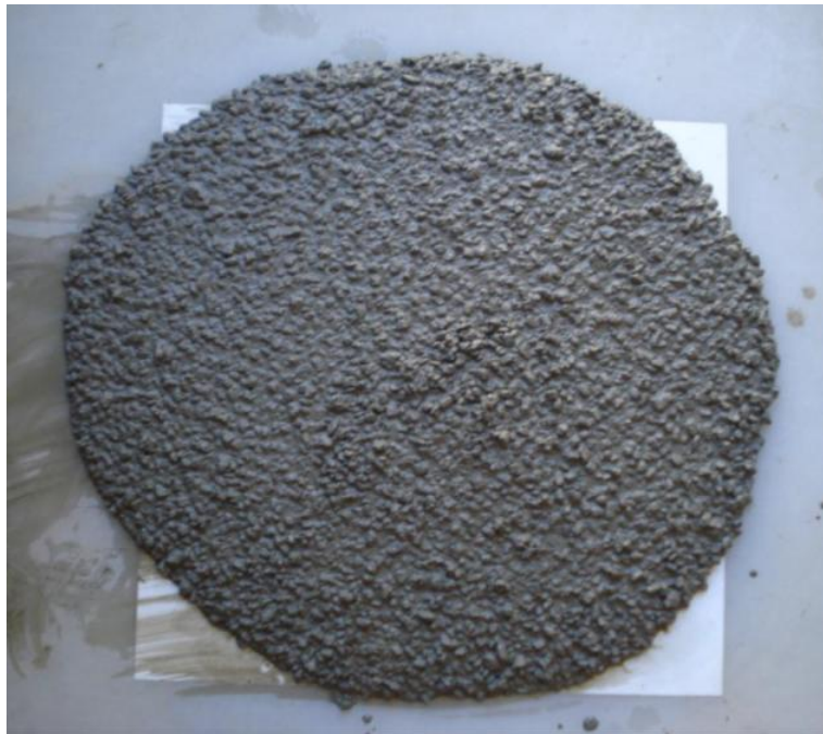
Figure 4.13: Slump flow of final HSS mixture
