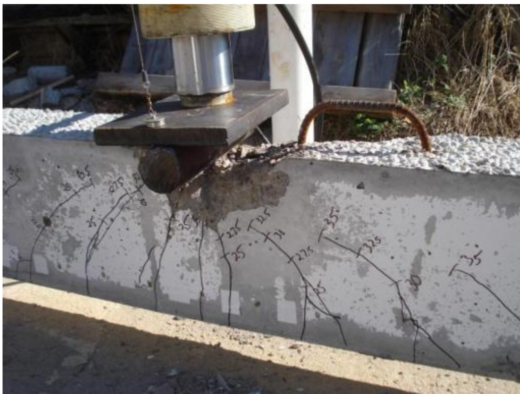
Figure 6.1: Cracking pattern of specimen NSC-1D
