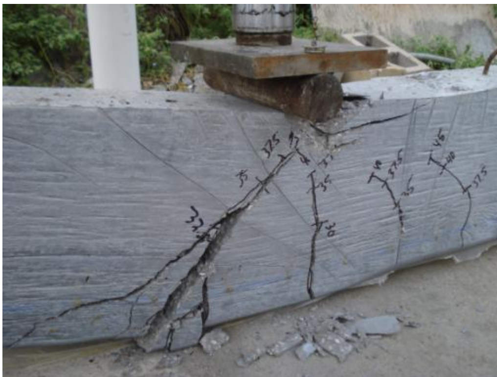
Figure 6.86: Cracking and failure of specimen HSL-1D
