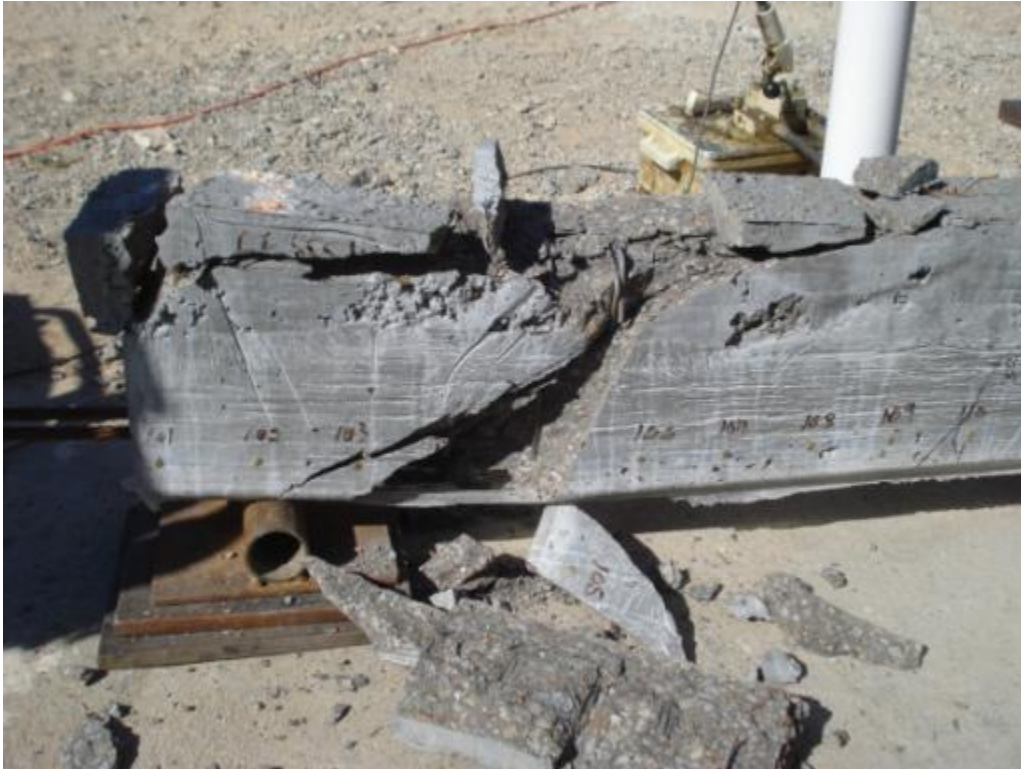
Figure 6.63: Shear failure of specimen HSC-3L
