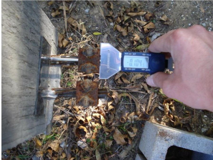
Figure 3.19: Measurement of strand end slip
