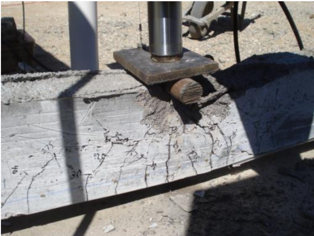
Figure 6.72: Cracking and failure of specimen HSS-1L
