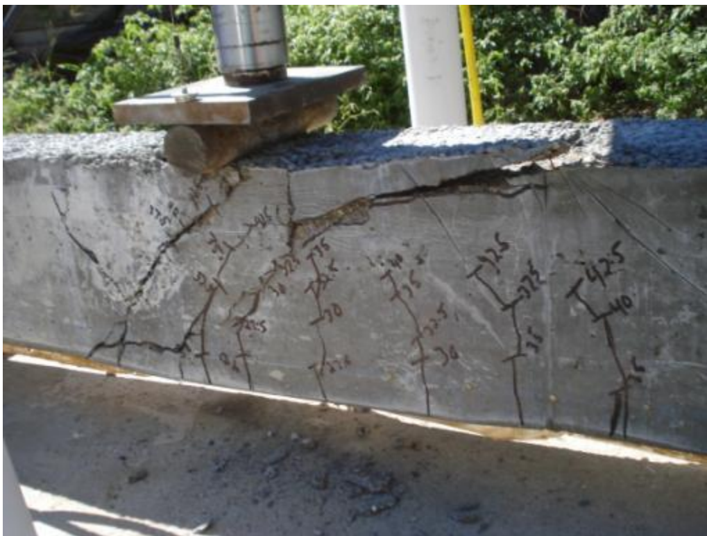
Figure 6.53: Cracking and failure of specimen HSC-1D
