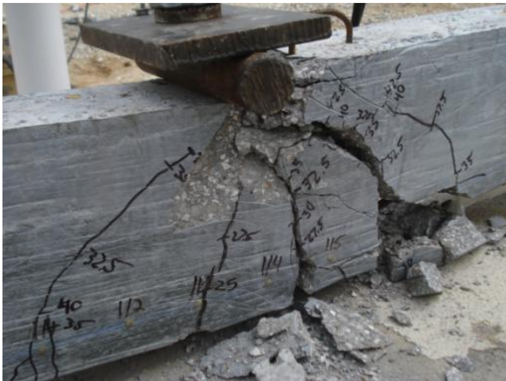
Figure 6.88: Cracking and failure of specimen HSL-1L
