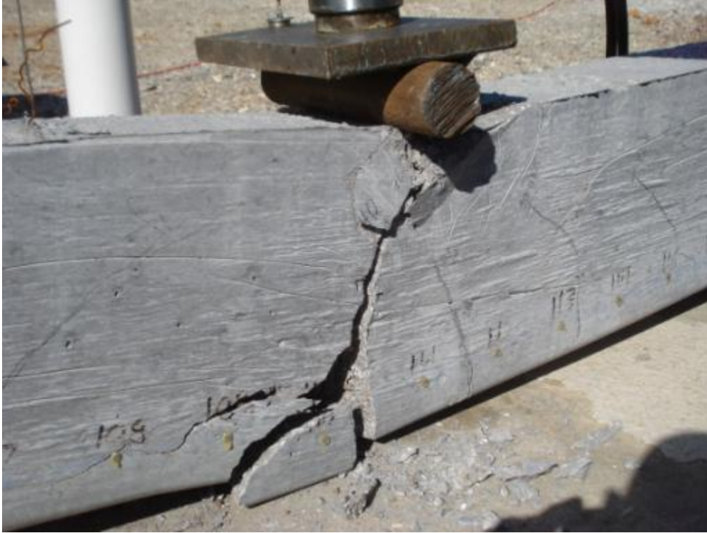
Figure 6.99: Cracking and failure of specimen HSL-4L
