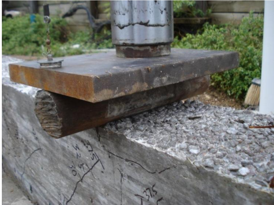
Figure 3.22: Application of point load for flexural testing
