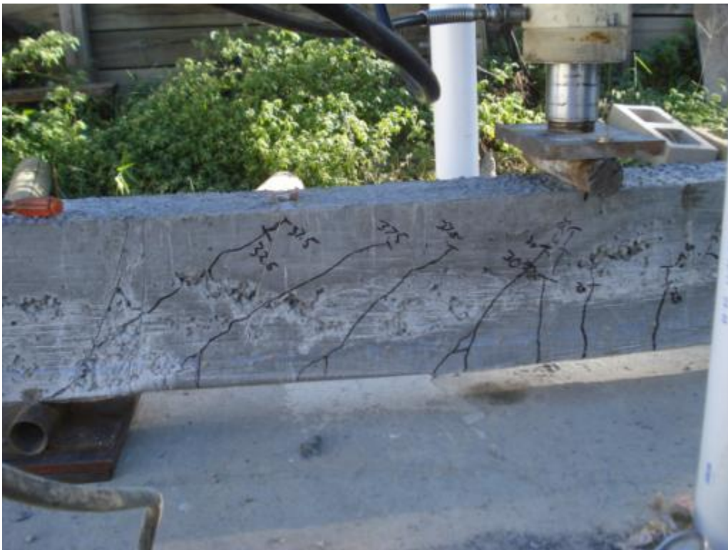
Figure 6.61: Cracking and failure of specimen HSC-3D
