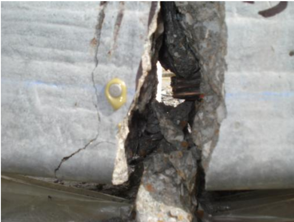
Figure 6.96: Strand fracture at failure of specimen HSL-3L
