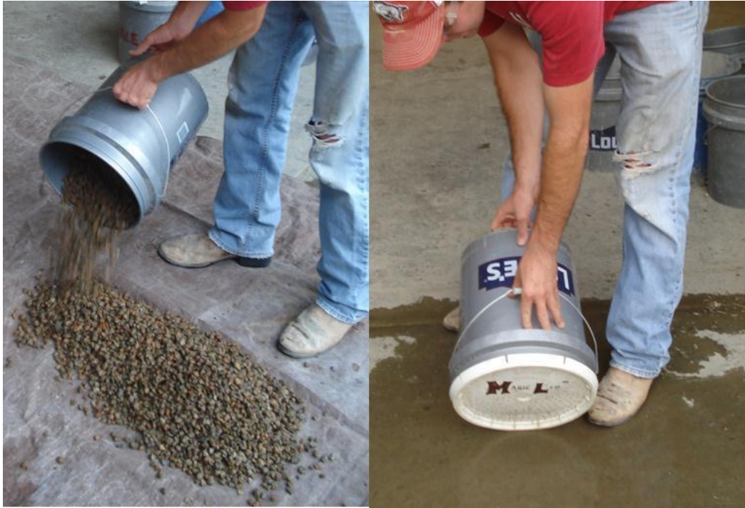
Figure 3.5: Aggregate preparation using tarp and perforated bucket lid
