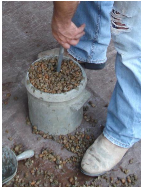
Figure 3.7: Performance of aggregate unit weight
