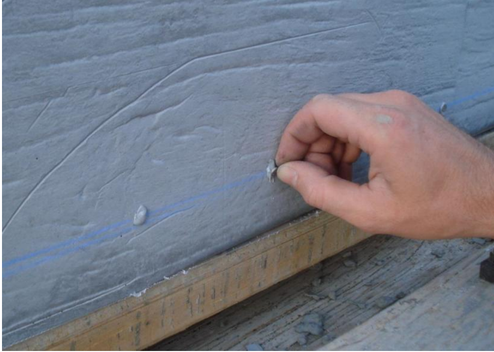
Figure 3.16: Placement of DEMEC points using epoxy
