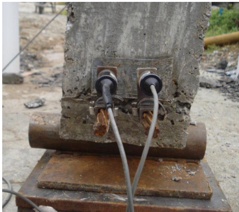
Figure 3.23: Placement of LVDTs to measure strand slip during flexural testing plate to the strong floor. All instruments were monitored continuously throughout each test with measurements recorded every second using a data acquisition system.
