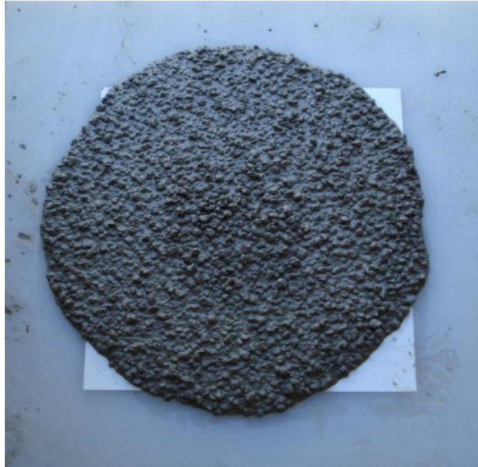
Figure 3.10: Adequate slump flow
