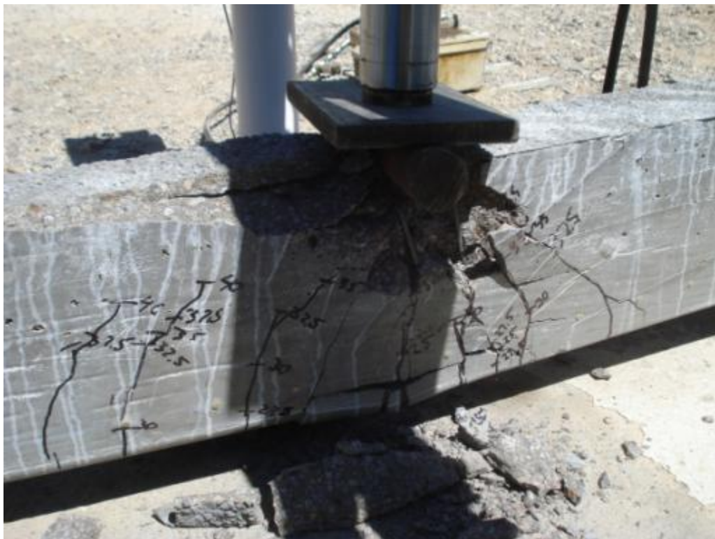
Figure 6.58: Cracking and failure of specimen HSC-2D
