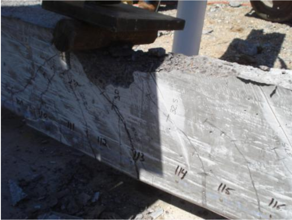
Figure 6.79: Cracking and failure of specimen HSS-3L
