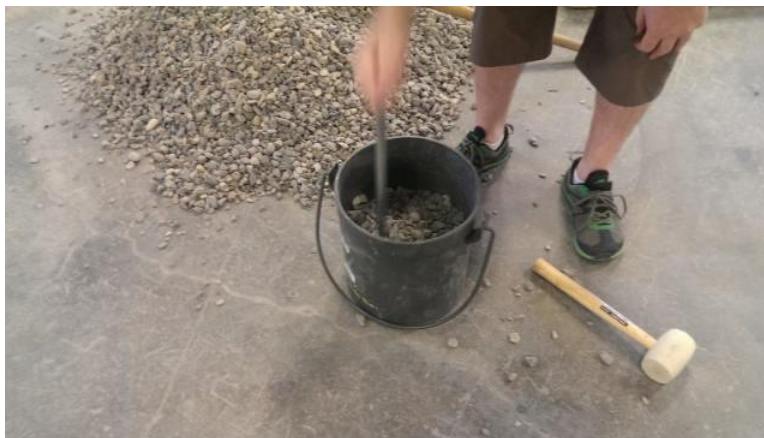
Figure 70 - Each lift is rodded 25 times.
