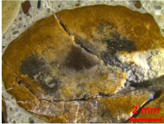
Figure 1 – ASR damage in chert coarse aggregate.
