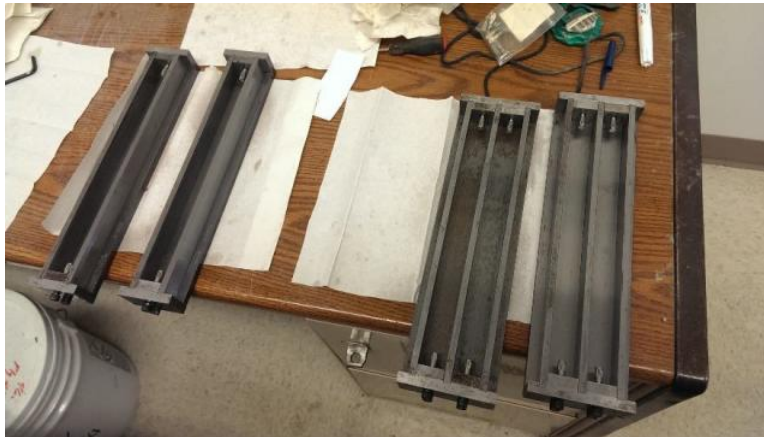
Figure 45 - Assembled molds ready for mortar
