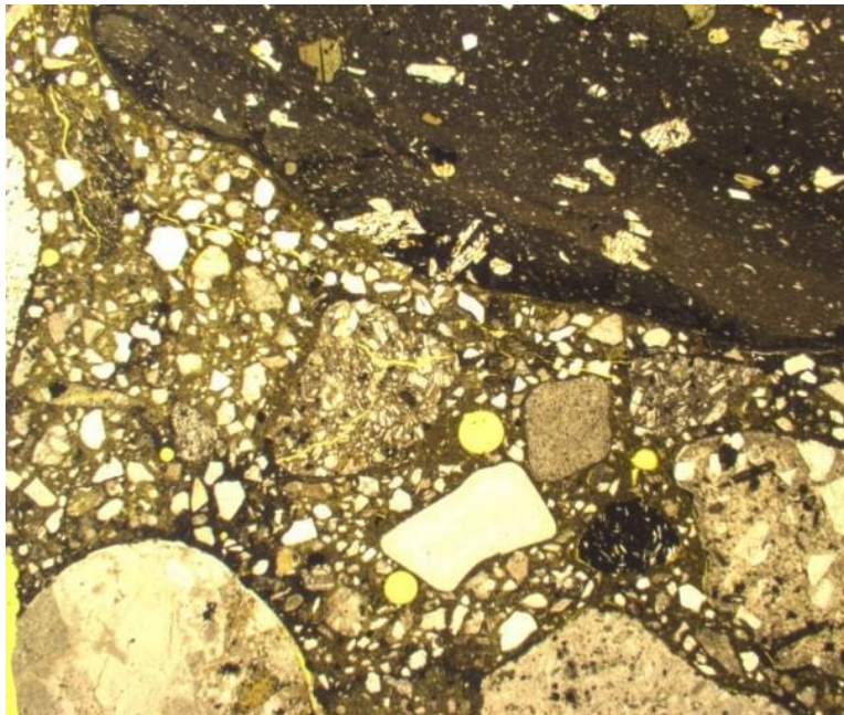
Figure 2: Concrete sample – the same area as in Figure 1. Plane polarized light. Magnification x12.5.
