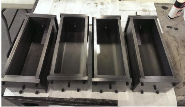
Figure 94 - 4-inch square prism molds ready for casting
