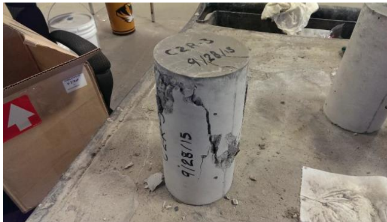
Figure 93 - Fractured cylinder after testing
