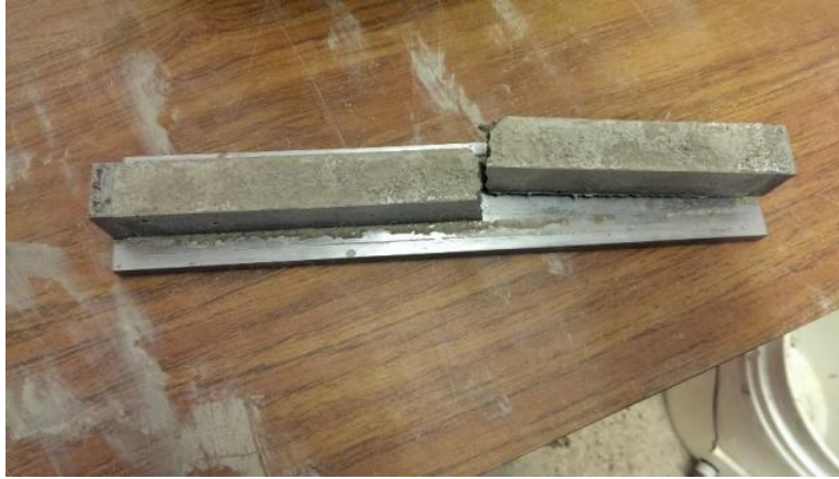
Figure 50 – This mortar bar broke during extraction
