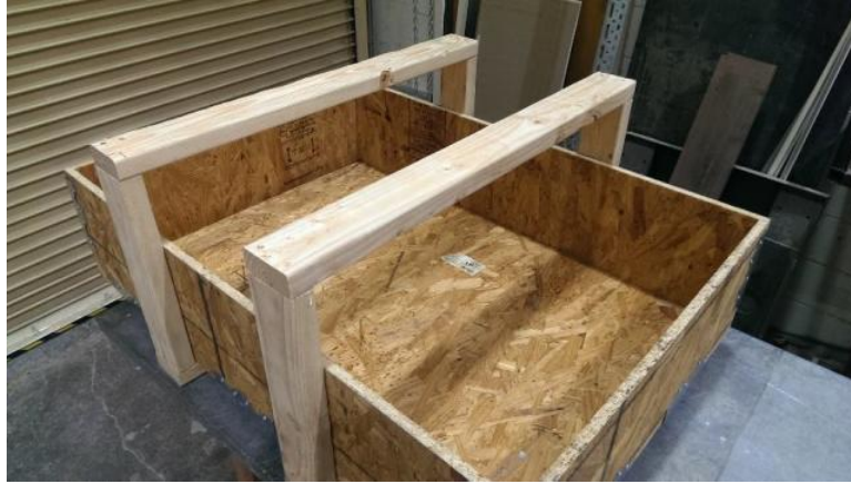
Figure 26 – Example shear specimen formwork
