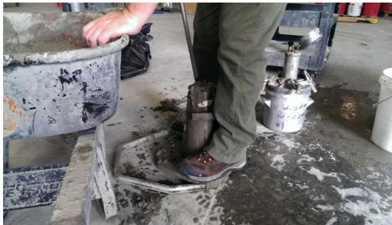
Figure 80 – The slump mold is filled in three layers, each tamped 25 times.
