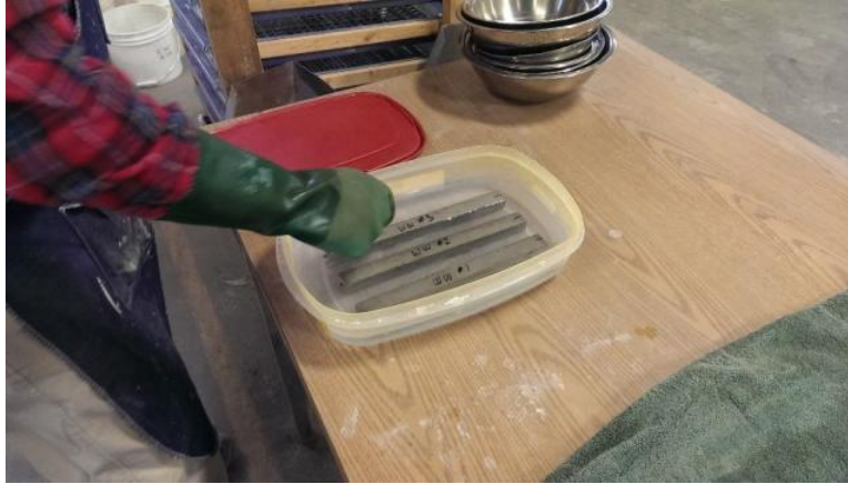
Figure 52 - After zero readings, bars were placed in 1N aqueous NaOH.
