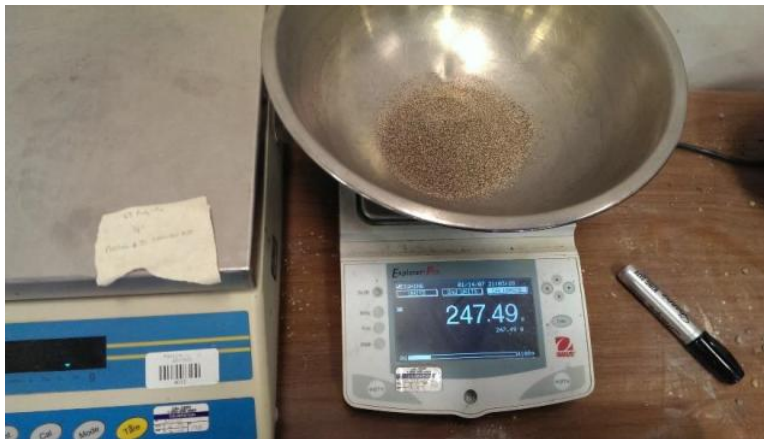
Figure 43 - Balance used to weigh dried aggregate
