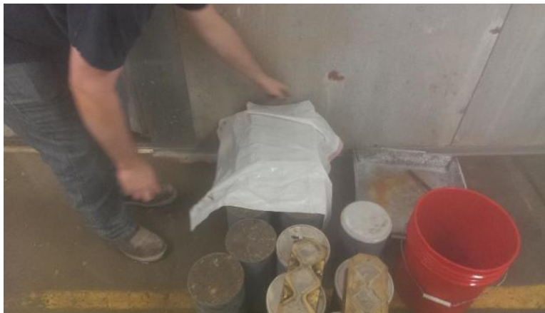
Figure 49 - Mortar bars placed in curing room and covered with plastic
