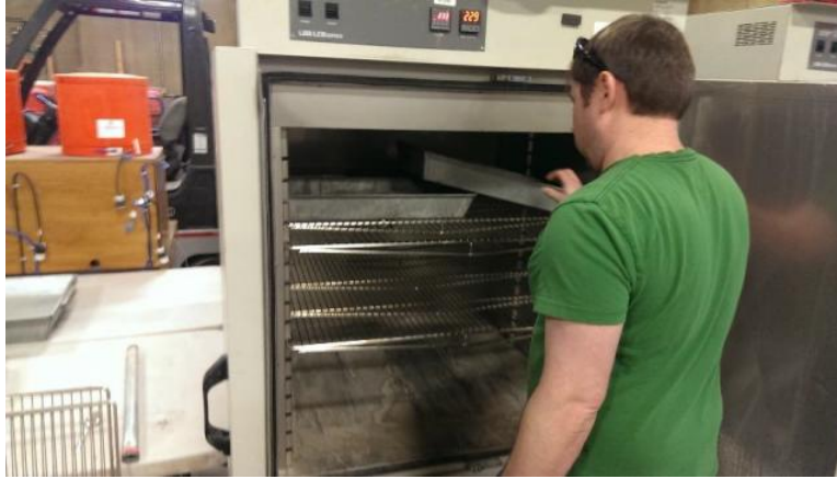
Figure 42 – Dana Schwartz of Fall Line placing washed material in drying oven.
