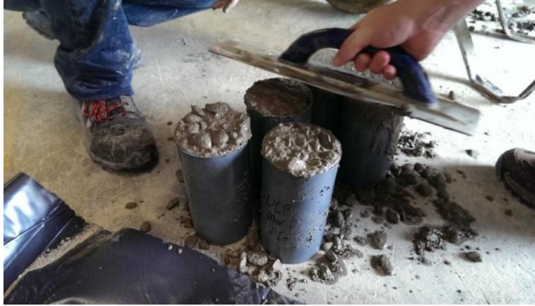
Figure 88 - Striking off cylinder molds
