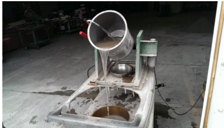
Figure 71- Washing aggregate in preparation for sieve analysis
