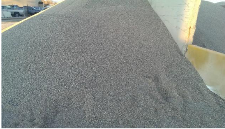
Figure 37 - 3/8" Gravel storage bin at Grand Junction Ready Mix
