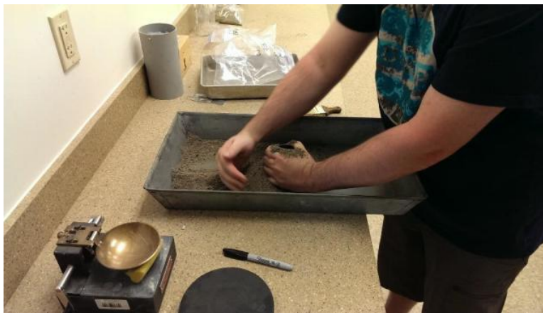
Figure 64 - Filling cone mold to check surface moisture of fine aggregate.
