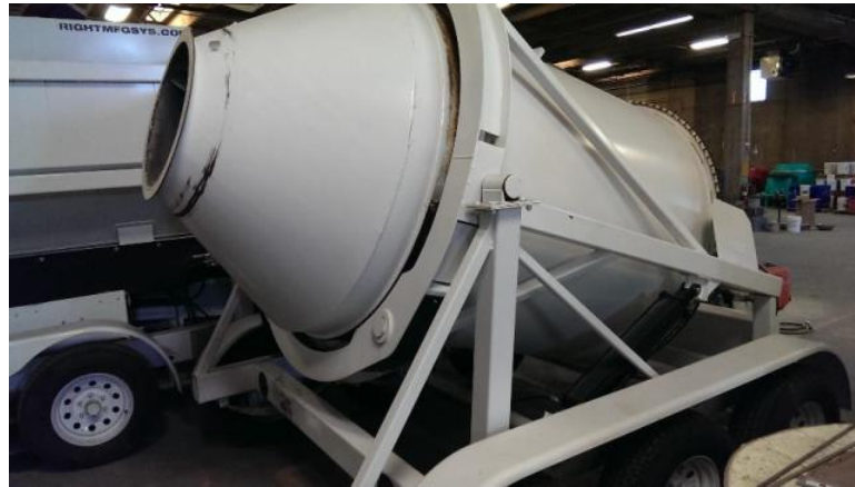
Figure 28 - The three-cubic yard mixer at Fall Line
