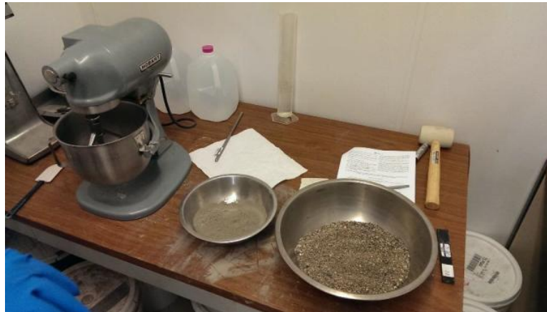
Figure 46 – Mixer with measured cement, water, and aggregate
