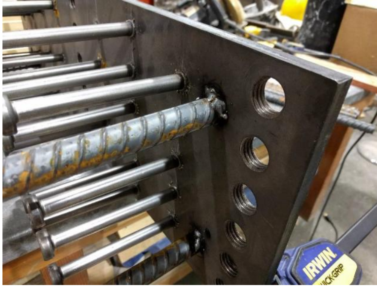
Figure 25 - MIG-welded joint between #6 rebar and sample end plates.
