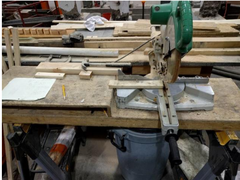
Figure 19 - Cutting wooden blocks for the welding jig.
