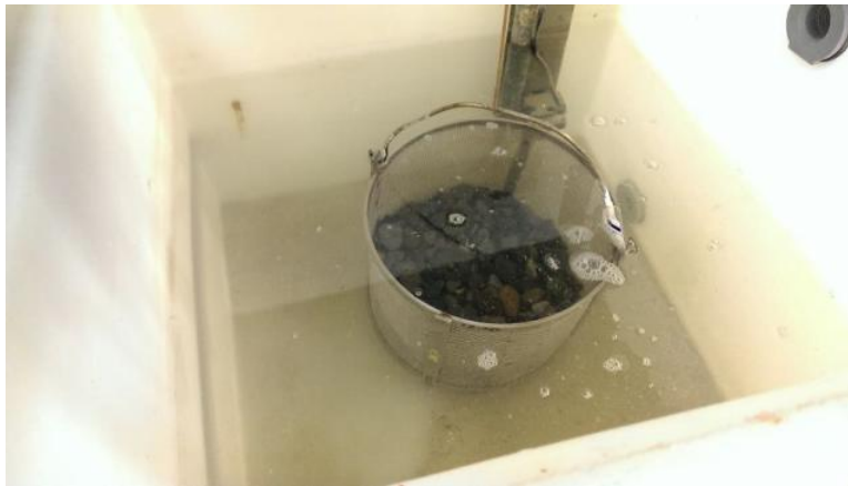
Figure 63 - Aggregate is immersed and weighed a second time. This apparatus allows the same scale to be used for both weighings.
