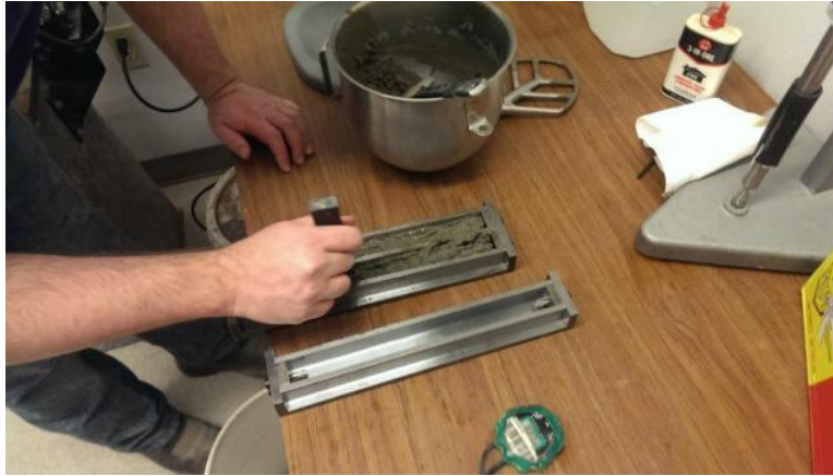
Figure 48 - Tamping mortar into molds
