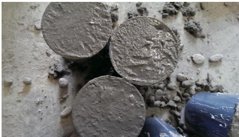
Figure 89 - Cylinders were allowed to rest 30 minutes before capping. Notice minimal bleeding.
