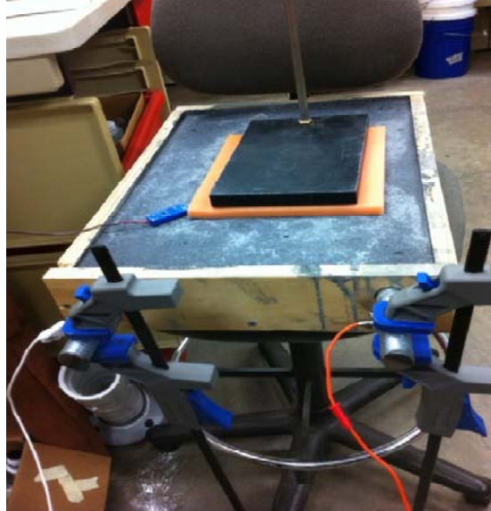
Figure 6.4: Small scale mat under testing conditions (Osweiler, 2012)
