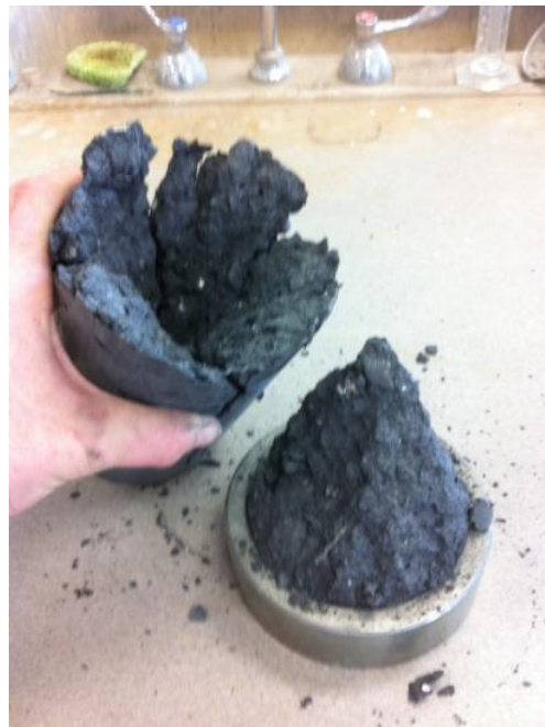
Figure 3.5: Preliminary conductive concrete workability (Osweiler, 2012)
