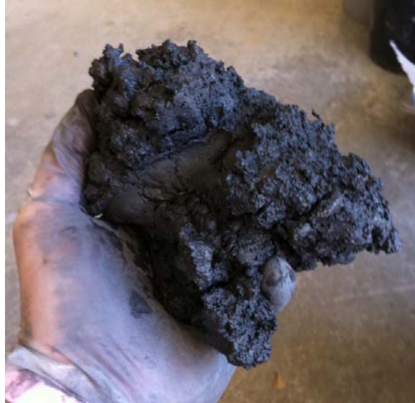
Figure 3.5: Preliminary conductive concrete workability (Osweiler, 2012)
