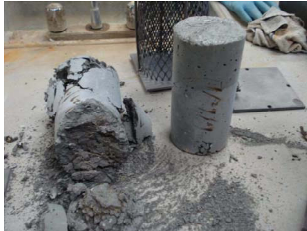
Figure 2.5: Effects of fire and rapid heating rates on conventional concrete (Hale, 2010).
