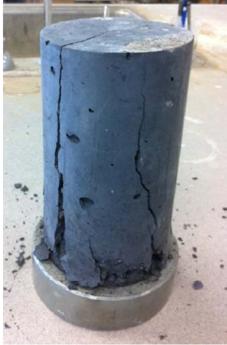
Figure 3.7: Compressive test results for Trial Mix 2 (Osweiler, 2012)
