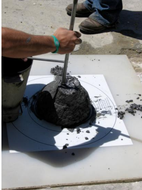
Figure 6.12: Slump of 4” for test mat 3 (Osweiler, 2012)
