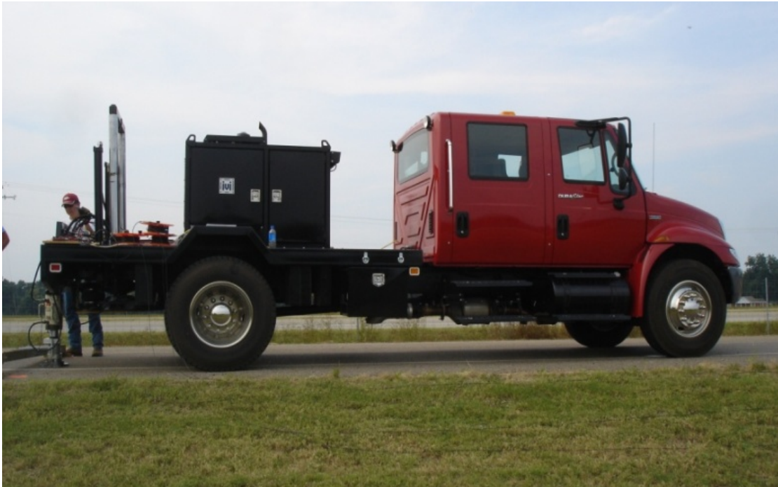
Figure 5.6. University of Arkansas vibroseis truck.
