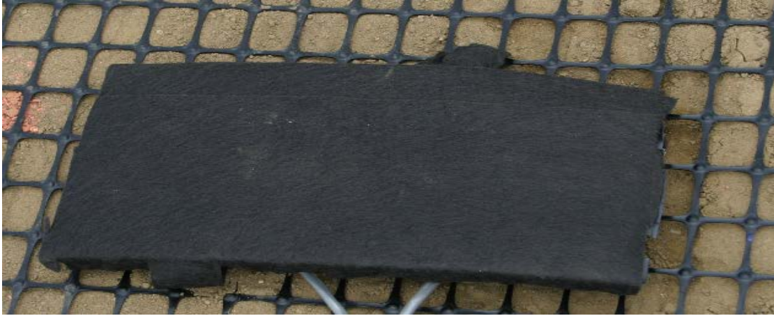
Figure 3.13. Geogrid strain gage protection, strip drain (Howard 2006).
