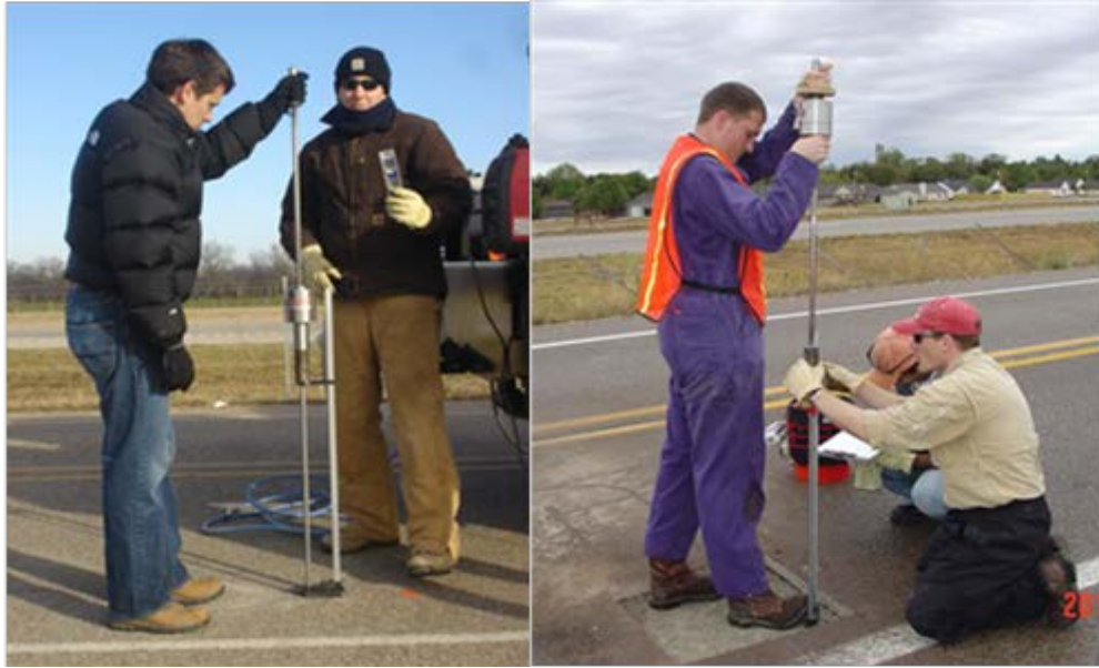
Figure 6.23. DCP testing at the Marked Tree site on December 2009 and October 2010, respectively.
