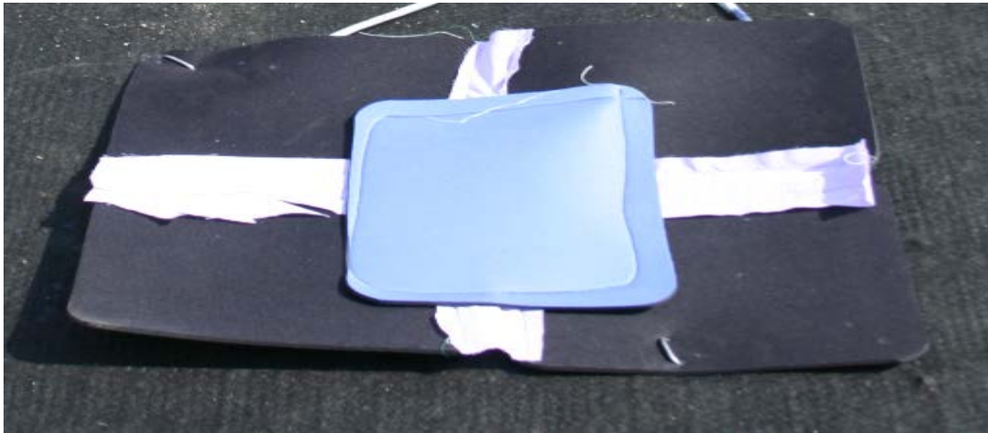
Figure 3.14. Geotextile strain gage protection, neoprene pad (Howard 2006).
