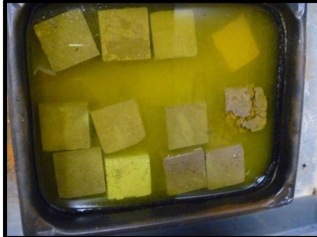
Figure 47: Concrete Specimens in Molten Salt Bath (John, 2012)
