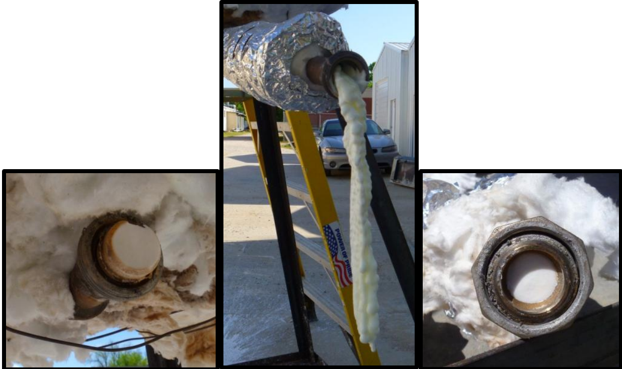
Figure 67: Salt Frozen in Lines during Testing
