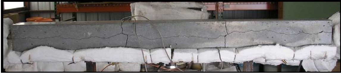
Figure 8: Cracking in Concrete Block with No Soft Material at Interface of Concrete and Stainless Steel Heat Exchanger (Skinner et al., 2011)
