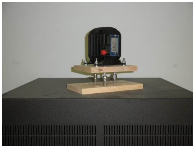
Figure 2.2. Final tactile transducer setup (Photo by K. Grimmelman)
