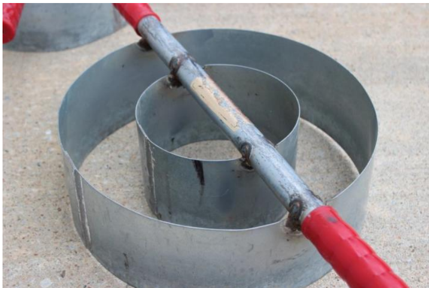
Figure 4.3. Photograph of a double-ring infiltrometer used in the study, manufactured by Turftec International. The diameter of the inside ring is 15.24 cm (6 in), and the diameter of the outer ring is 30.5 cm (12 in). The height of the ring is 10.2 cm (4 in).
