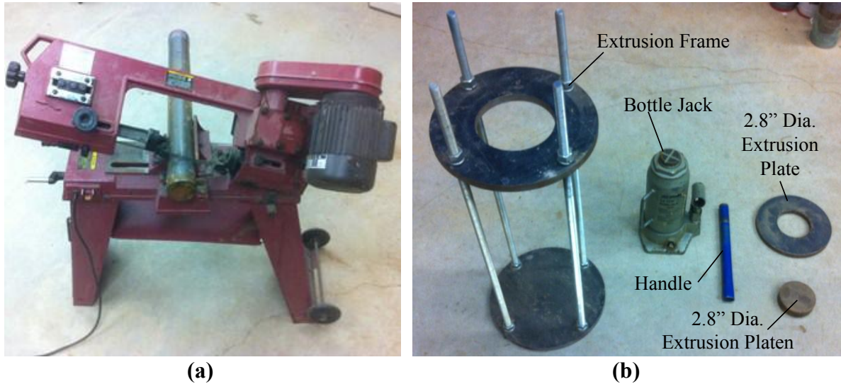
Figure 3.37. (a) Band saw used for cutting Shelby tubes, and (b) 12-ton hydraulic bottle jack apparatus used for extruding samples.
