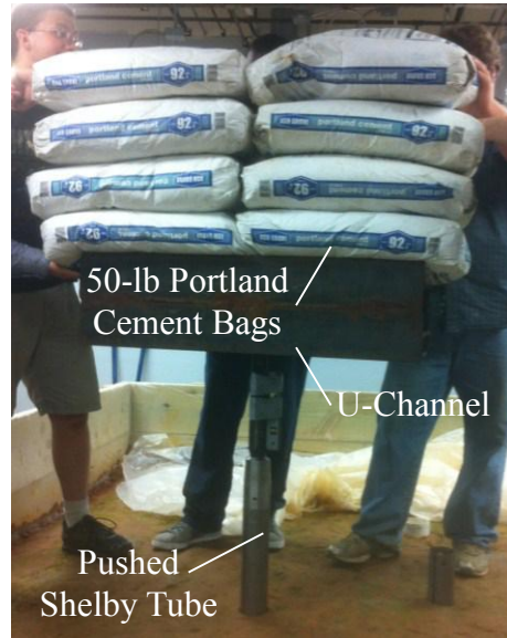
Figure 3.31. Shelby tube pushed into Test Pad 2.
