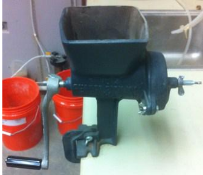
Figure 3.40. Photo of No. F-4 Quaker City Grinding Mill used for grinding soil samples.
