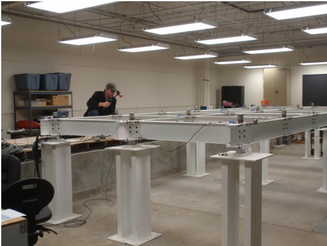
Figure 3.26: Impact testing with instrumented hammer at node B1 of the grid model structure. Photo taken by Dr. Kirk Grimmelsman
