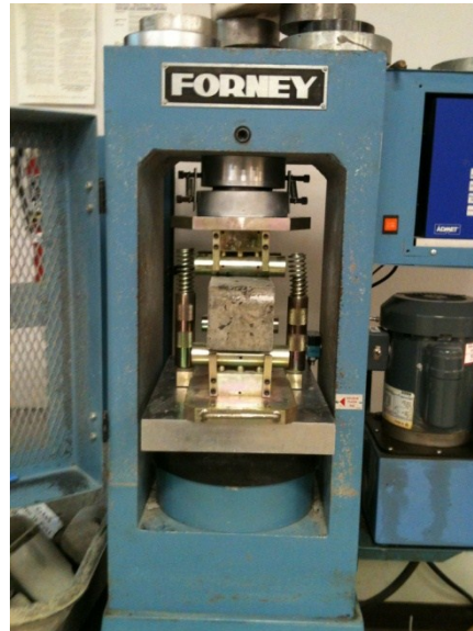
Figure 3.5.3.1. Modulus of rupture testing device with specimen.
