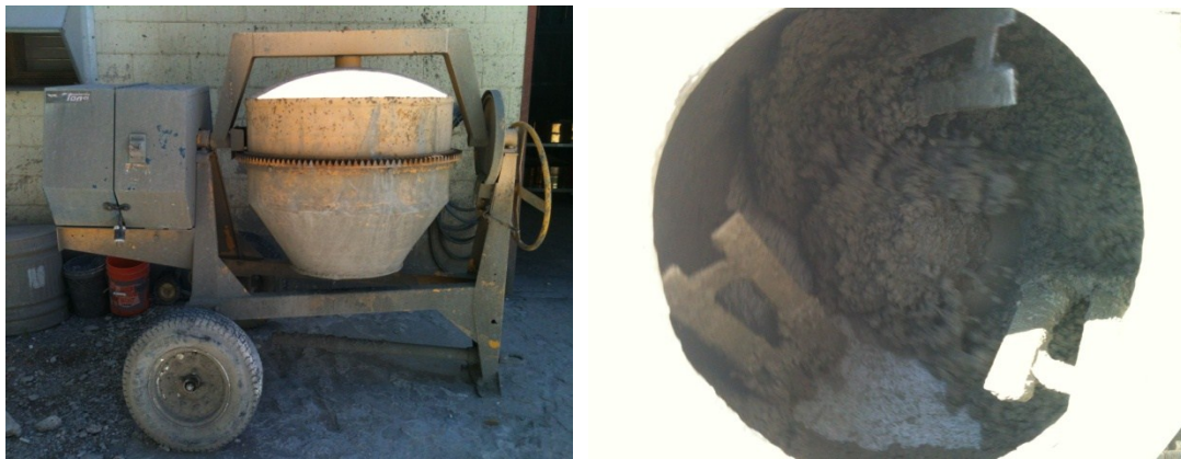
Figure 3.3.2. Concrete mixer and the mixing concrete.
