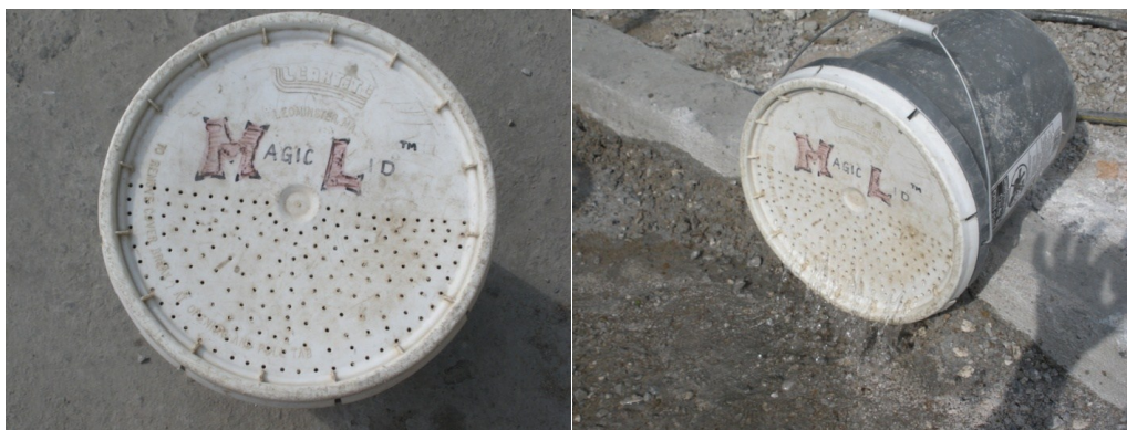
Figure 3.3.1. Removal of excess water after soaking duration for LWA.
