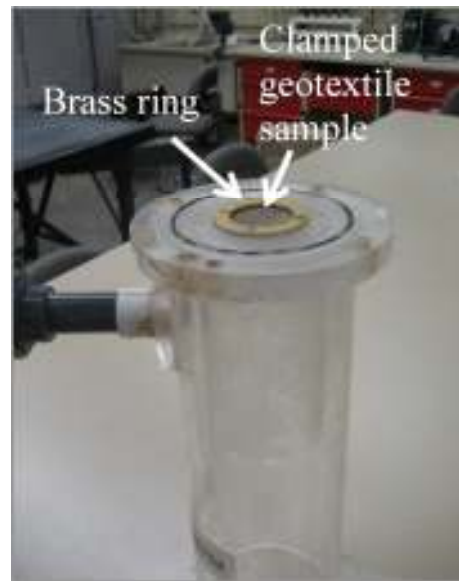
Figure 3.41. Geotextile sample secured using brass plate in the permeability device.
