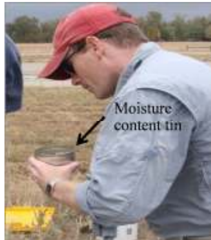
Figure 3.12. Base course moisture content sample.
