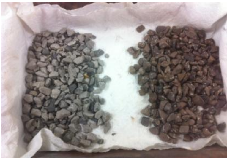
Figure 6.3: Sandstone before (left) and after (right) 500 hours at 550°C
