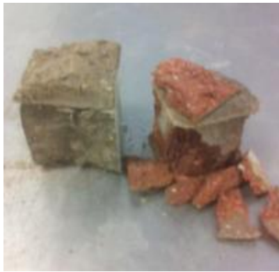
Figure 6.6: Concrete cube before (left) and after (right) 500 hours at 585°C
