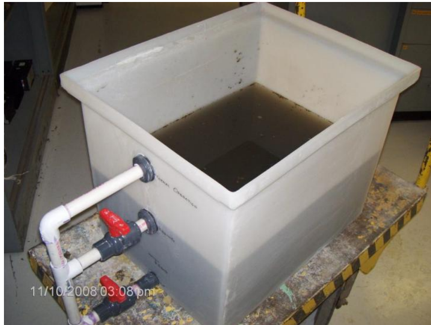
Figure 5.2: Initial aerated batch system mussel laboratory microcosm.
