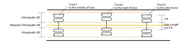
Figure 47 Geometrical definition of wheel path based on traffic wandering
