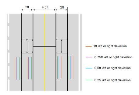
Figure 17 Schematic of marking reference lines
