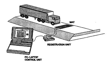
Figure 7 Sensing measurements with a mat (Blab and Lizka 1995)
