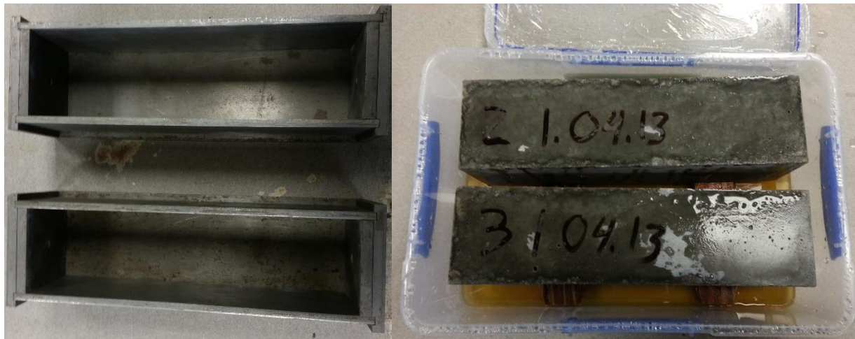
Figure 2.6. Typical CPT prism molds (left), and storage containers (right). Picture used with permission from Richard Deschenes.
