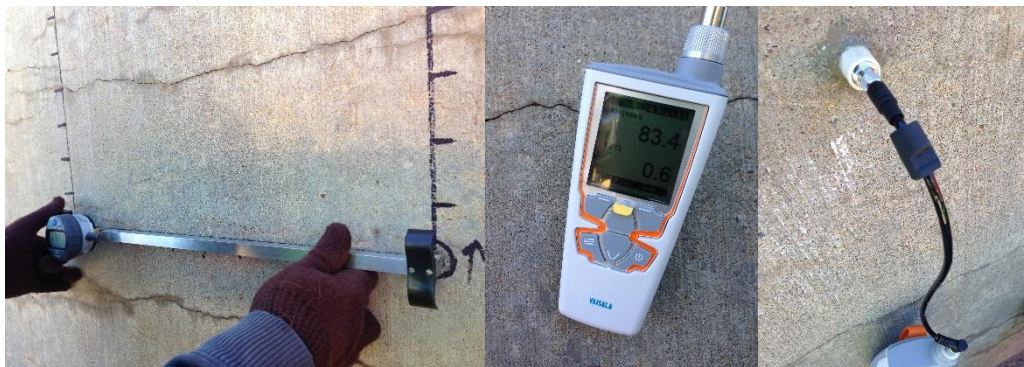
Figure 2.9. DEMEC gage during length-change measurement (left), portable humidity indicator (center), and humidity probe inserted into a humidity port (right). Pictures used with permission from Richard Deschenes.
