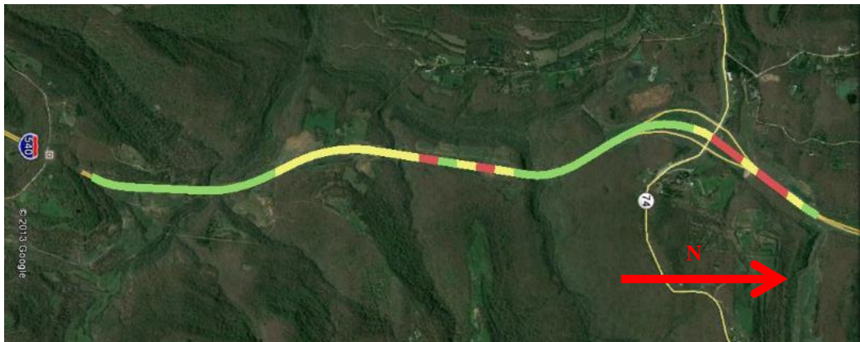
Figure 3.1. Median barrier damage level along Interstate 49. Figure produced in Google Earth.
