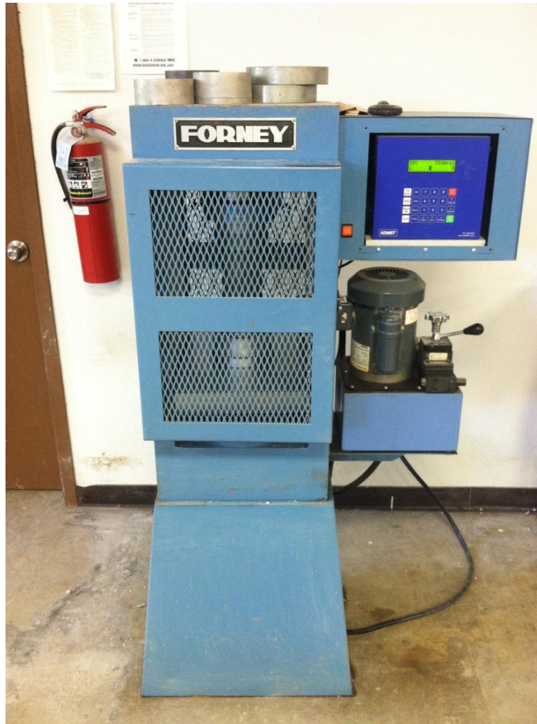
Figure 3.5 Concrete Testing Machine
