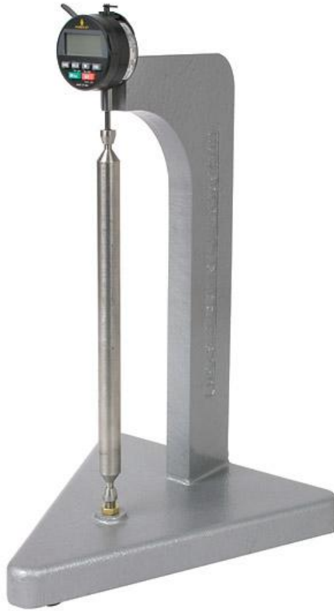
Figure 3.4 Length Comparator with Digital Indicator ( www.humboldtmg.com )
