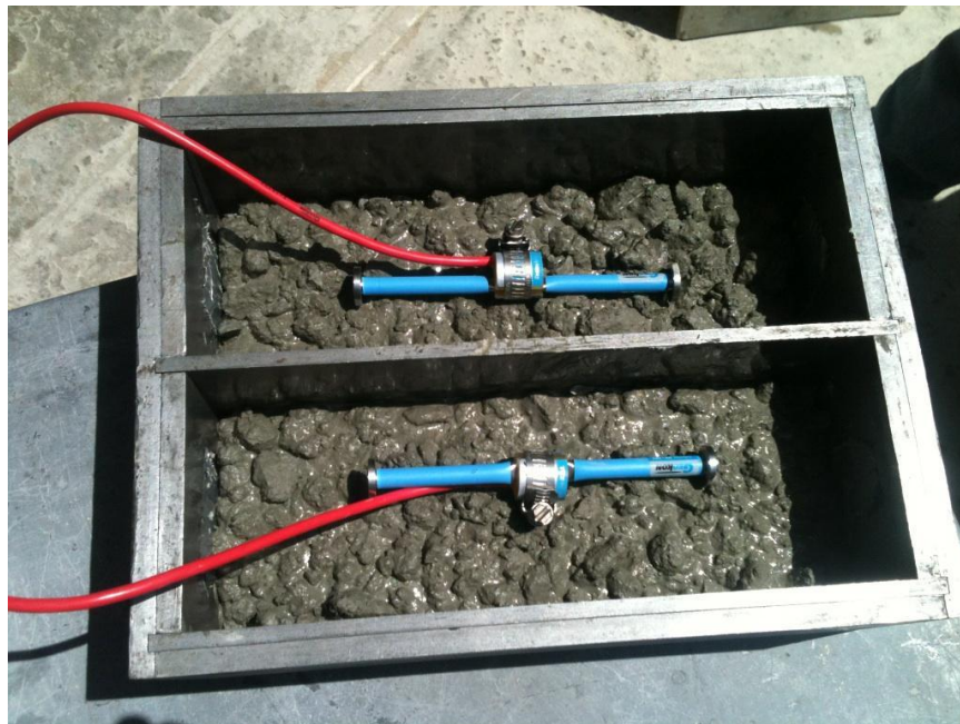
Figure 3.6 Vibrating Wire Strain Gage Placement in Steel Molds
