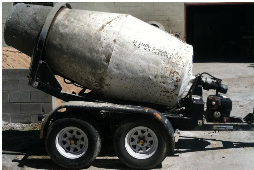
Figure 3.10 One Cubic Yard Rotating Drum Mixer
