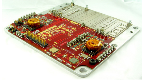
Figure 12. Single phase MCPM SOI/SiC prototype inverter.
