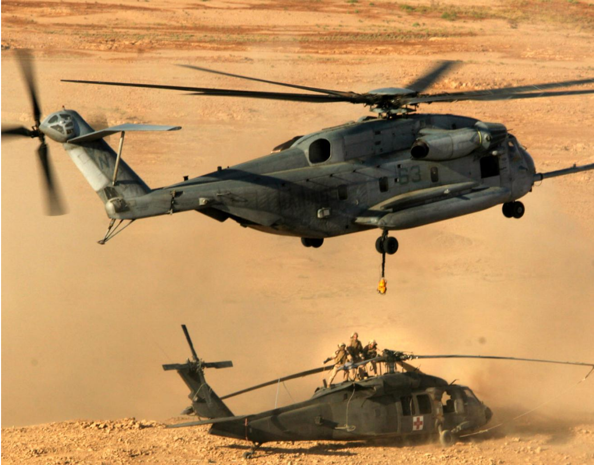
Figure 1 – A helicopter in flight prepares to lift another helicopter after being stranded. The rotor blades of the helicopter are deformed by extremely large amounts. These blades are acting as loaded cantilever beams with the anchor point at the hub of the rotor.
