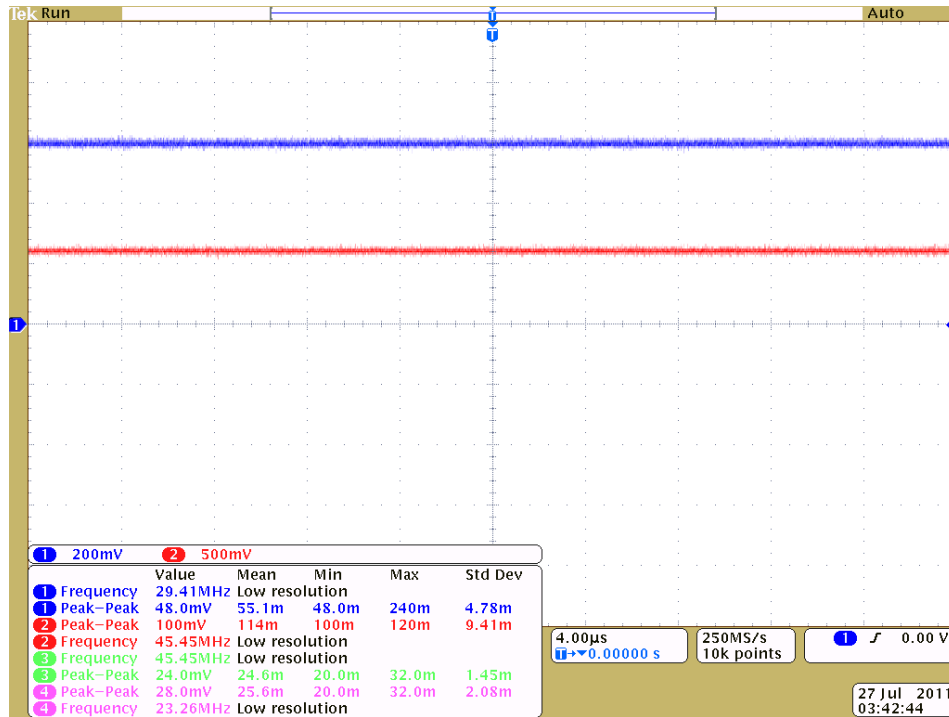
Figure 6.6. Output voltages under 0 to 1.2 V input sweep with negative output scale changed to 500 mV.
