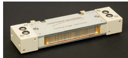
Figure 1.2. High power laser diode array manufactured by Northrop Grumman Cutting Edge Optonics. The array is based on vertical stack of 36 MCCs.
