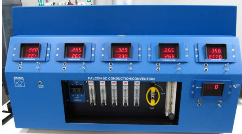
Figure 2.2. Picture of Sikama 5-zone reflow oven.
