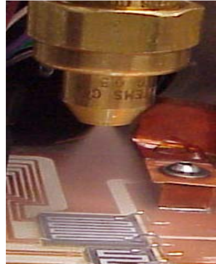
Figure 1.3. Picture of a thermal test heater being spray cooled.
