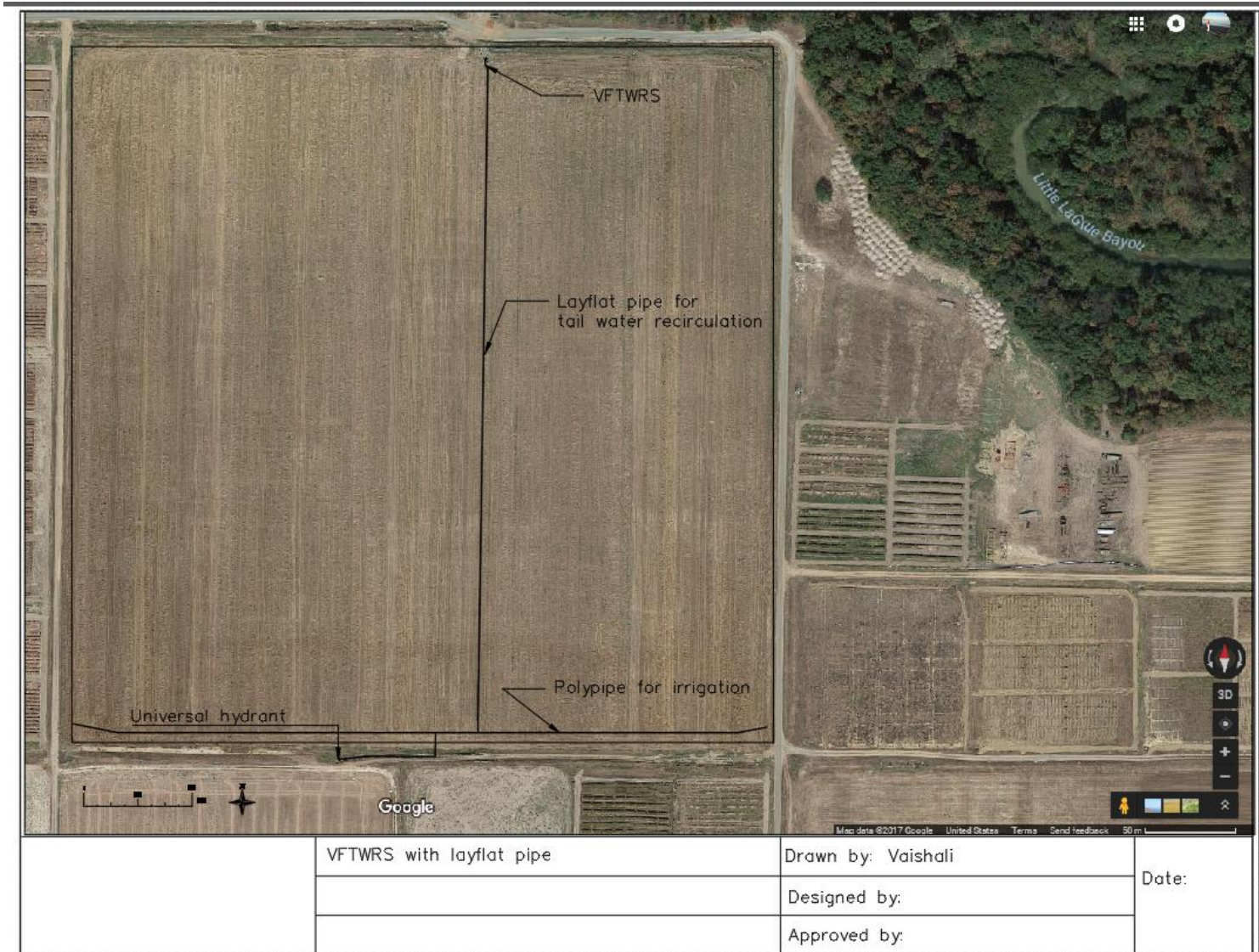
Figure A.2: Plan for Scenario 1 (VFTWRS-Grid with lay-flat pipe)
