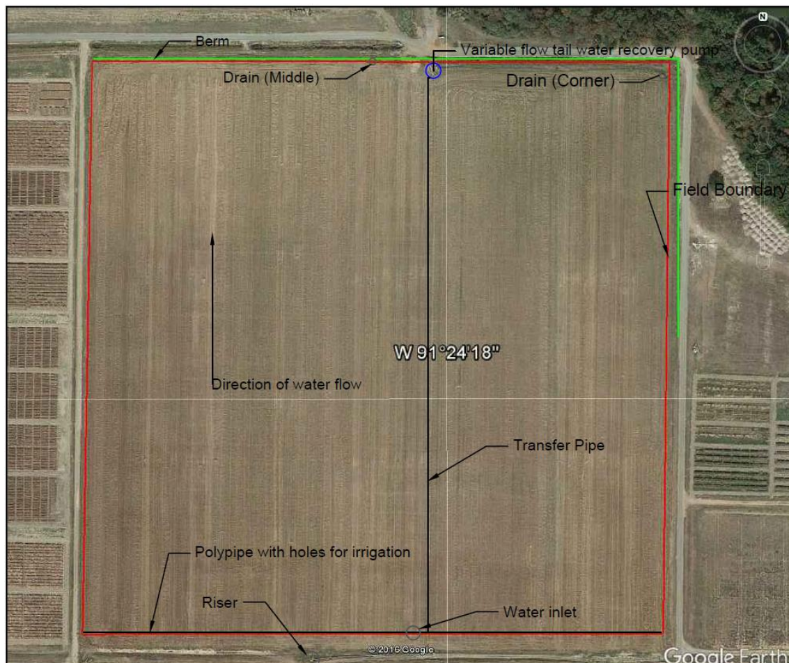
Figure 2.1: Overhead view of the VFTWRS in the experimental field.
