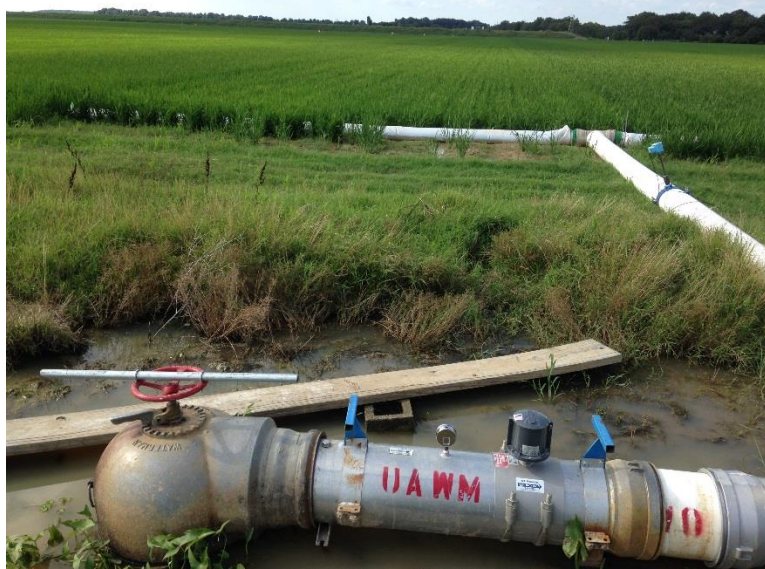
Figure 3.4: Universal hydrant is connect to a propeller flowmeter, a badger meter and a pipeline which supplies water to the field
