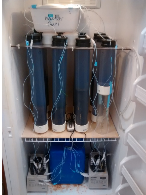
Figure 6: ICI experimental setup, with aerated amended water reservoir lower middle, pumps on either side of it, cores above supported with acrylic rack, and outflow receptacle on top, all within incubator.
