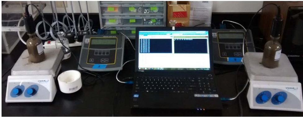
Figure 7: \dot{N}_{\text{sed}} testing station, showing laptop computer (center), YSI 5100 DO probes, 300mL BOD bottles, and stir plates.
