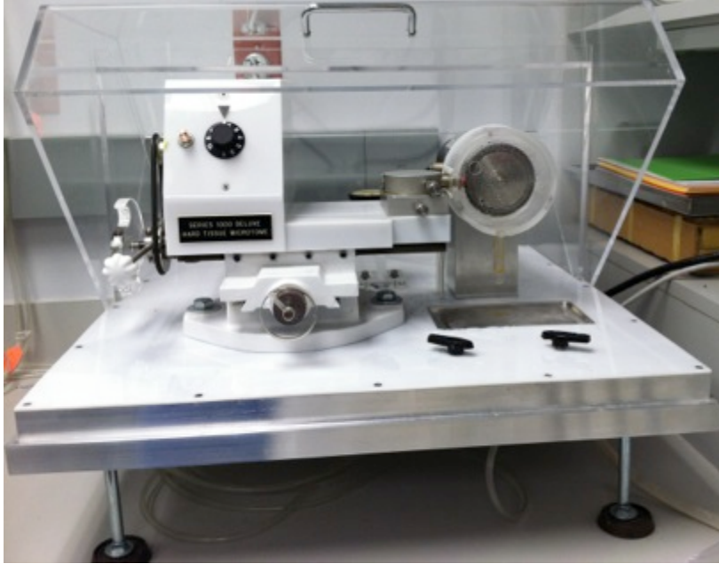
Figure 8 Hard tissue microtome used to obtain longitudinal sections bucco-lingually of all teeth
