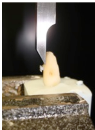
Figure 11. Debonding in the Universal Testing Machine
