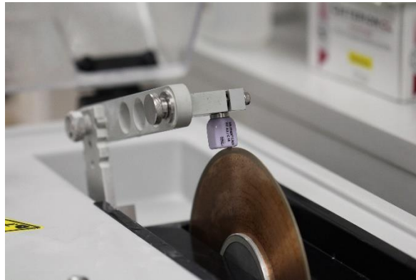
Figure 4. Blade IsoMet Wafering Blade-15LC, 7in
