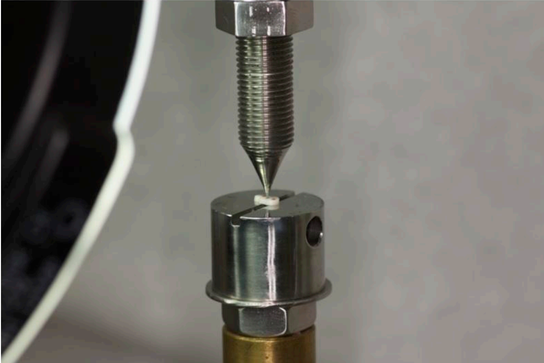
Figure 7: Loading each slice with the MTS plunger. Each slice was positioned so as to contact only the apical aspect of the post on the loading
