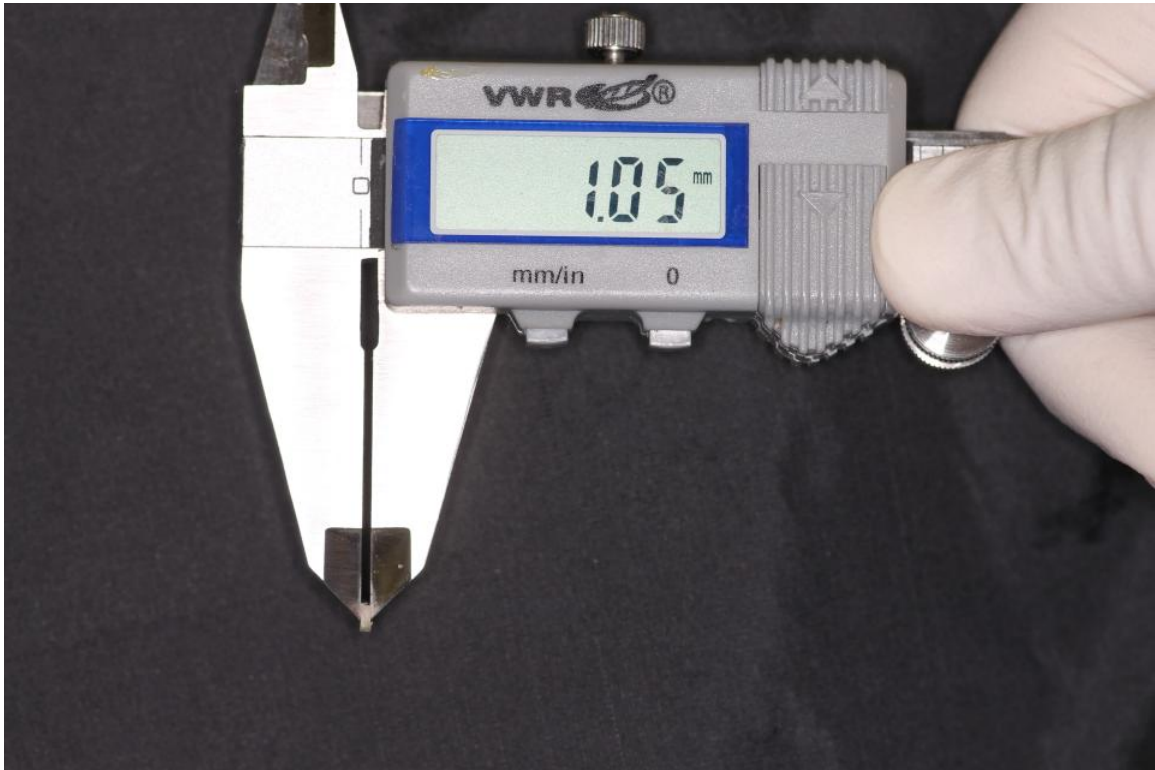
Figure 5: Digital caliper used to measure the thickness of each slice
