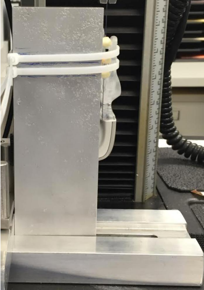
Figure 10. Cable ties holding AccelDent in place against the teeth.
