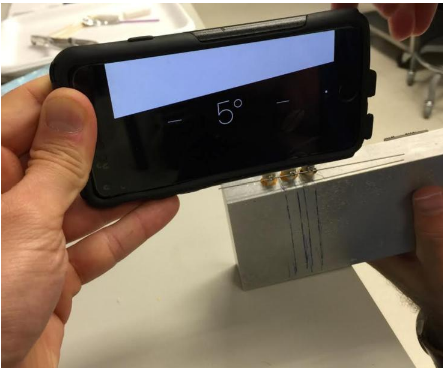
Figure 13. Bracket angulation confirmed with iPhone 6 level.
