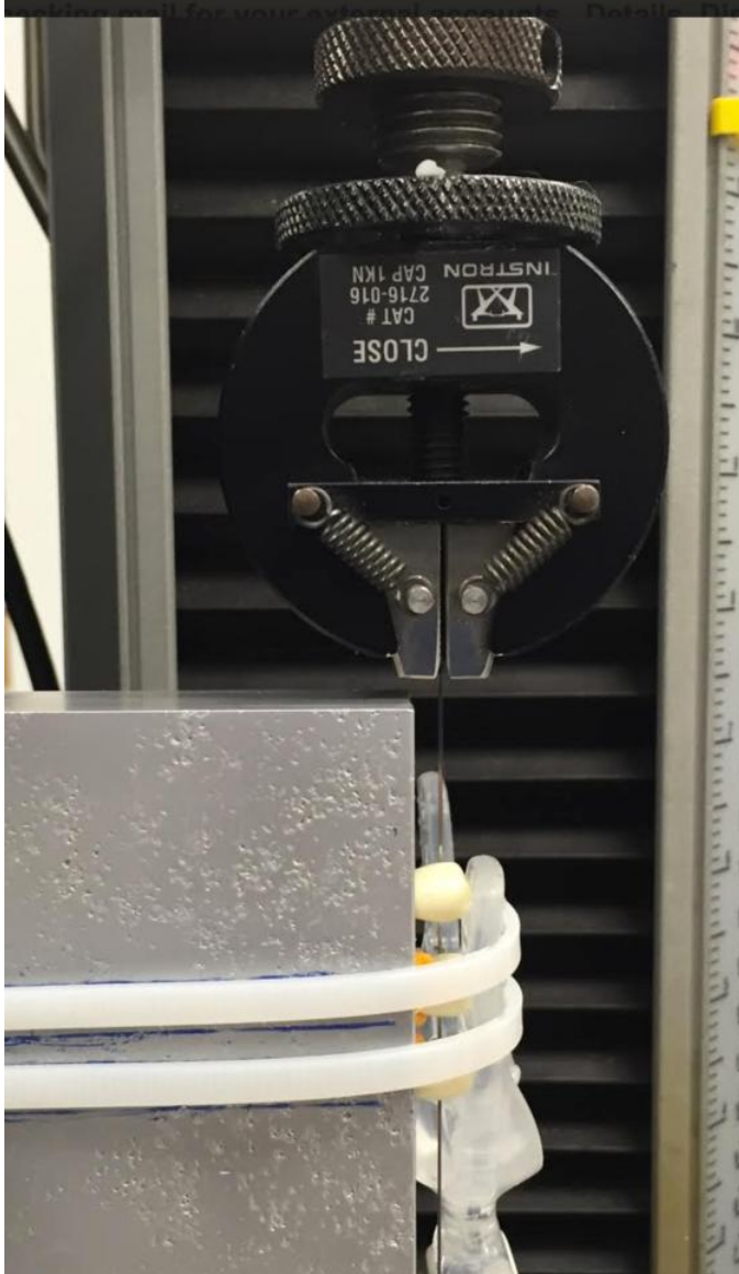
Figure 12. Vice grip tightened with composite ball marker in place.
