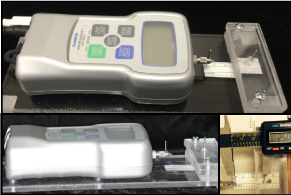
Figure 3. Shimpo force gauge test stand with fixed distance of 25 mm
