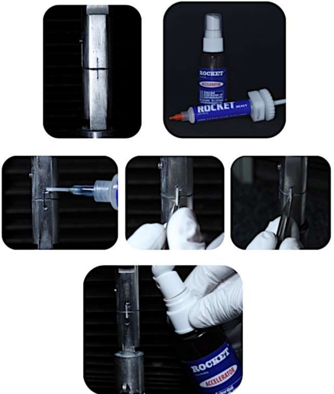
Figure 15. Sample attachment to the metal fixture using cyanoacrylate glue
