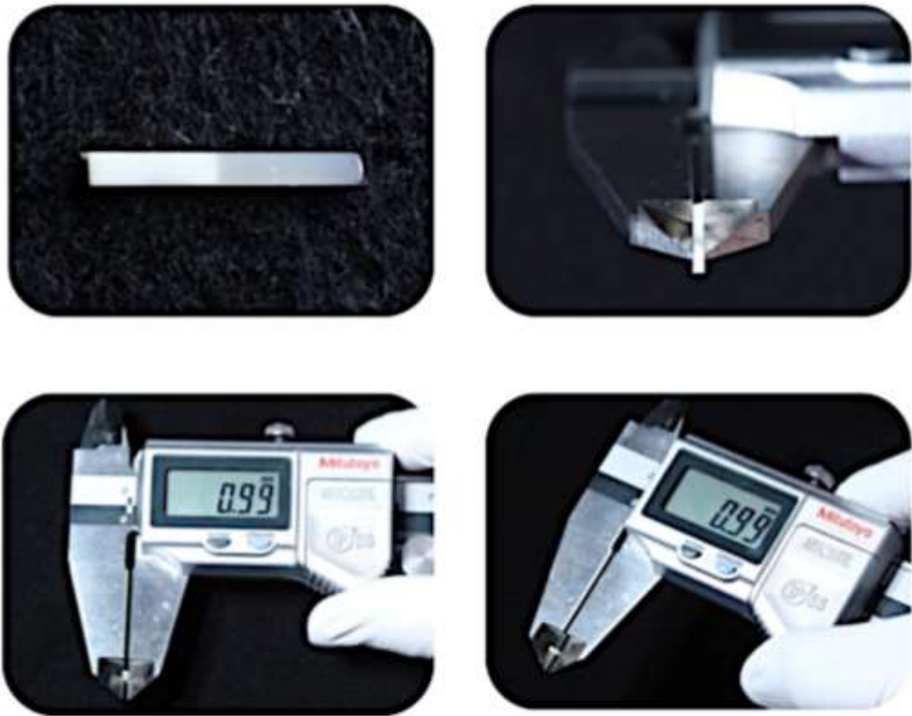
Samples width and thickness measurement at the composite/dentin interface using digital caliper Absolute IP66 (Mitutoyo, Aurora, Illinois)
