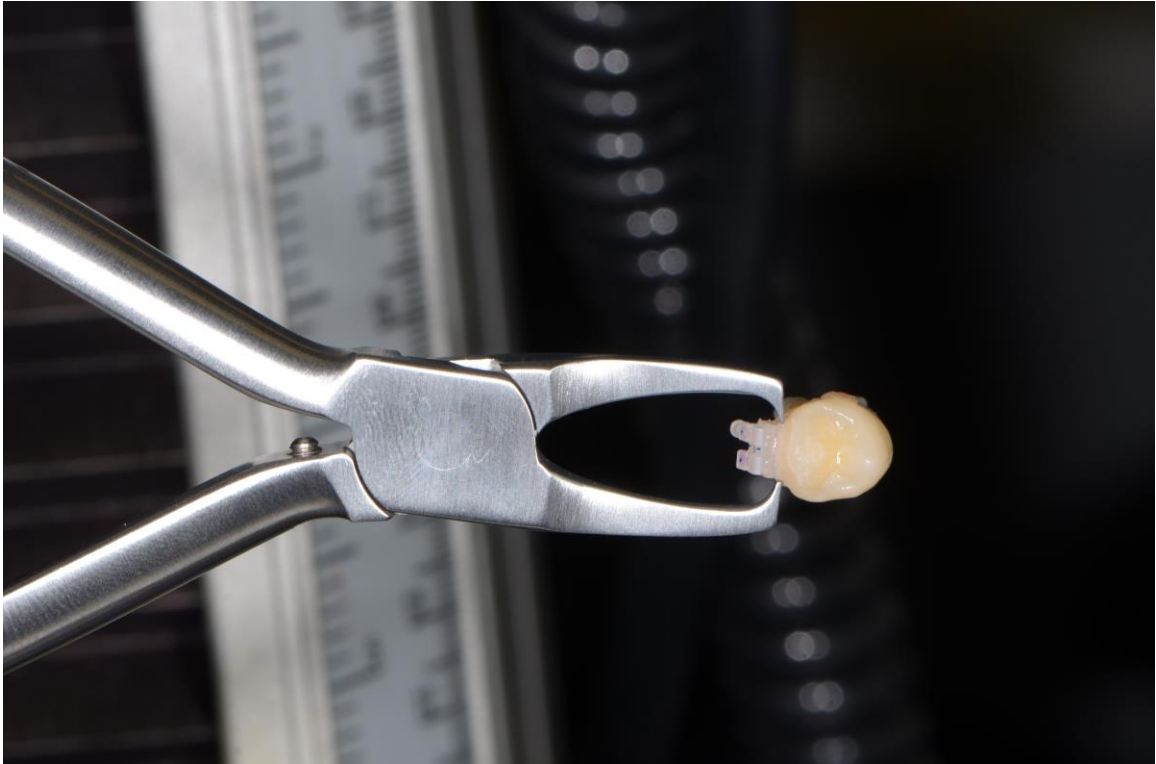
Figure 7. Samples placed in the Straight Bracket Removing Plier in a mesiodistal direction.
