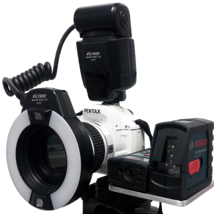
Figure 4: Camera setup for taking standardized photographs. Pentax Camera with ring flash mounted with a laser distance measure device and laser level atop a tripod.
