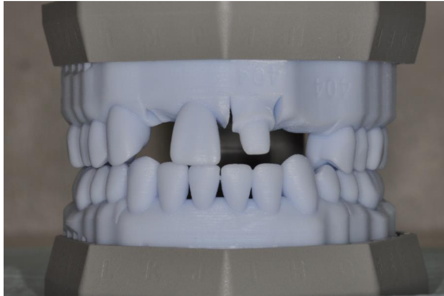
Figure 10: The SLA cast with the trimmed die
