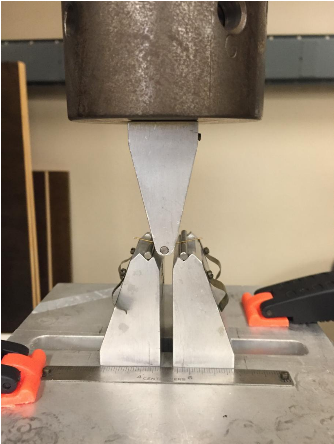
Figure 8. Instron Universal Testing Machine Performing Three-Point Bend Test
