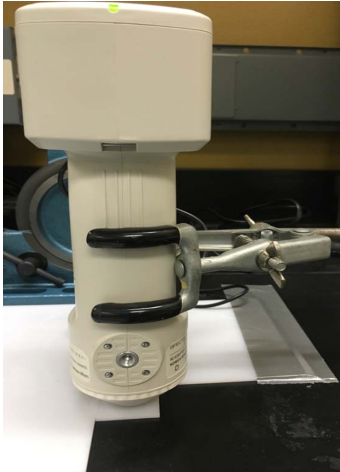
Figure 4. Color measurements were obtained with a spectrophotometer.
