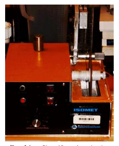
Figure 2: Isomet Diamond Saw used to section wires
