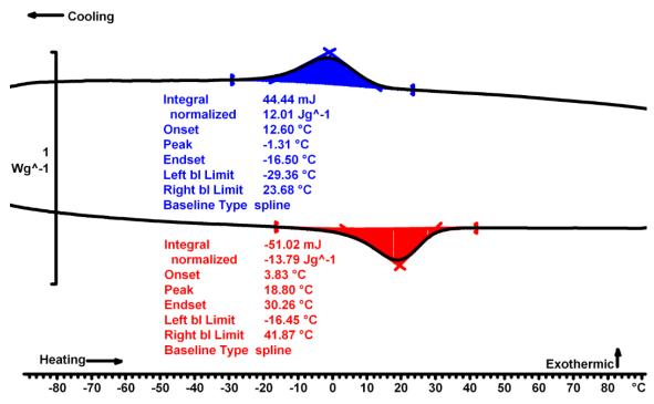
**Figure 5:** Example of DSC Thermogram Analysis
