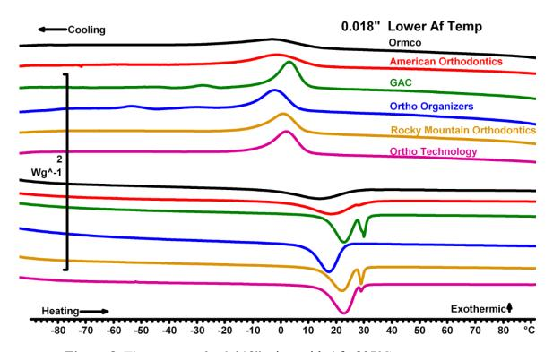
Figure 8: Thermogram for 0.018" wires with Af of 27°C
