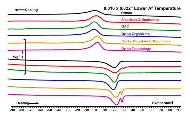
Figure 9: Thermogram for 0.016 x 0.022" wires with Af of 27°C
