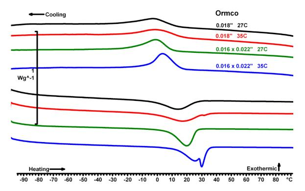
Figure 13: Thermogram for all variants of Ormco CuNiTi wires
