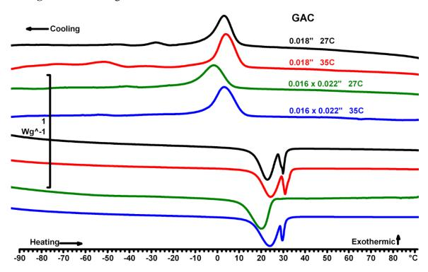
Figure 14: Thermogram for all variants of GAC CuNiTi wires
