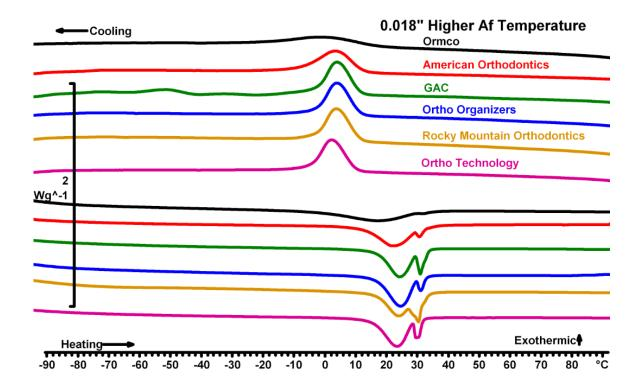
**Figure 7**: Thermogram for 0.018" wires with Af of 35°C
