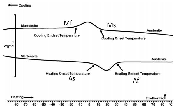
**Figure 1:** Example of DSC Thermogram
