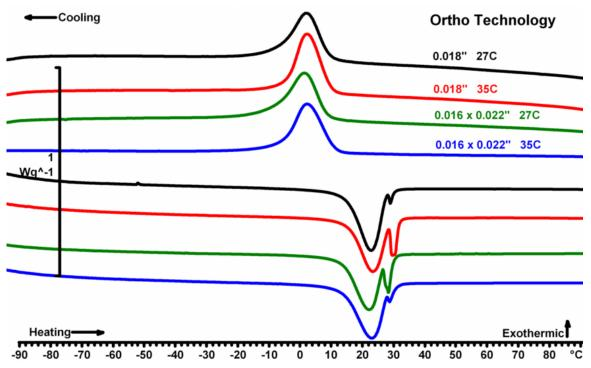
Figure 11: Thermogram for all variants of Ortho Technology CuNiTi wires
