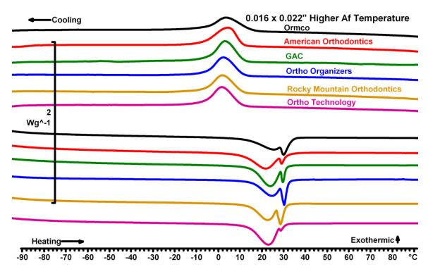
Figure 10: Thermogram for 0.016" x 0.022" wires with Af of 35°C
