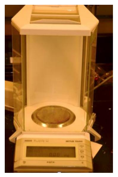
Figure 3: Scale used to measure wire segments
